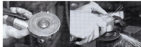
Chances are that the roller will be a little tight, and you will have to take a little off the inside of the sector shaft. Jim uses a small grinder that has been fitted with a soft wheel. Jim takes his time and removes only a little material, virtually polishing the area, and tries the roller and washers again.
