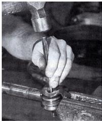
The pin is driven out of the sector shaft with a hammer and punch.
