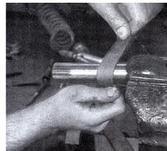
the shaft has deep pits or gouges, you need to have the shaft rechromed.
