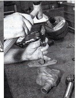
With the box clean, it is time to remove the old bushings. As this photo shows, the bushings are very thin. To get the old ones out, a screwdriver is gently tapped between the bushings and the wall of the box. And we mean gently. The trick is to pry away the edge just enough so a punch can be used to drive out the bushings. Be careful not to gouge the box in the process.
