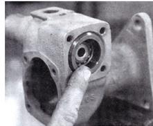
The lower bearing and race are greased and installed. CP also recommends that a few drops of 3 in 1 oil be used on the bearings.
