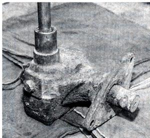
box is not in the center (straight) position. Use a pair of vise grips to spin it into position.
