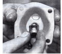
The washer slips into the notch in the end of the sector shaft, and the assembly is slid into place.
