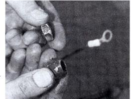
Some of the early boxes came with this star washer to hold the adjustment screw in place. Toss it. The problem is that the keyway in the screw allowed the fluid in the box to leak out. The CP kit includes a new non-keyway screw to alleviate this problem.
