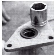
A socket is used to set the new rubber seal in place.
