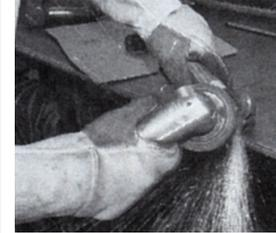
As the sector shaft needs to rotate, the welds need to be ground smooth so nothing is sticking out to catch on the inside of the housing.
