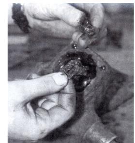
With the box secured in a vise, a hammer and brass punch is used to tap the sector shaft out. It does not take much effort to do this, so don't take a big swing with the hammer or you will flare open the end of the shaft.
