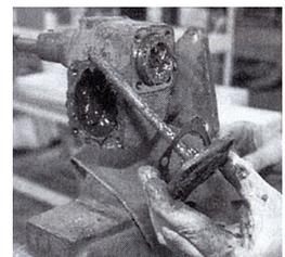
A few taps and the grease-covered worm gear assembly is out.
