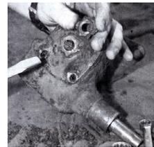
While the kit includes a new screw, it does not include the washer it screws onto. So when disassembling the box, be sure to keep it safe. With the cover off, it becomes apparent that this box has been filled with grease. It should have 90 weight gear oil in it. The problem is that the grease will cling to the walls of the box, and the gears will eventually be running dry. This will cause the gears to mar each other, especially in the center, of straight, position.
