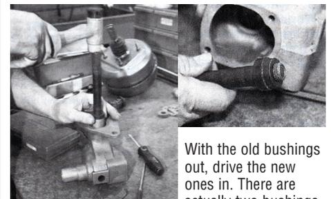
and they are driven in from the opposite ends of the box. Care is taken to drive the bushings in straight and square.
