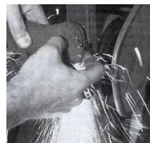
The pin is longer than necessary, and it will need to be ground down to fit. Holding the pin flush on one end, the other end is shortened using a sander.
