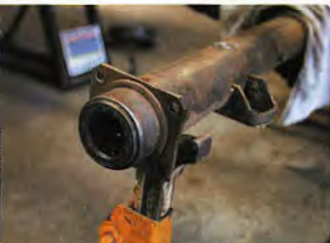
06 To complete the brakes, we installed CPP's 5-bug axle shafts, brake brackets, rotors and callipers for a killer, clean look. The custom-made calliper bracket is designed to mount directly to the backside at the axle flanges of the rear end using the provided hardware.
