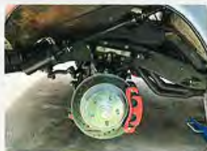
15 CPP's 6-piston brake calipers are a two-piece forged caliper design with six cross bolts for added strength. The piston sizes are staggered to minimize tapered pad wear, and it uses the same pads as the '97-'12 Corvette for an easy-to-find, cost-effective pad replacement.
