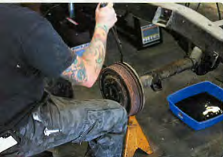
05 We will be swapping out the factory brakes for a new set from CPP, so the original hardware needs to be removed.
