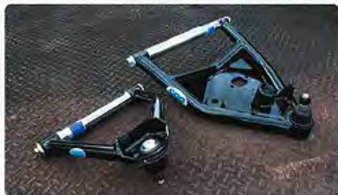
14 On this build we will be testing out Classic Performance Products all new Totally Tubular control arms and coilovers for a static yet adjustable suspension. After installing the lower control arms, upper control arms and coilovers, you can get a real feel for how well this system was designed. Fully adjustable, incredibly strong and engineered with a DIY mindset.
