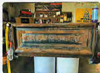
17 Jeff's unique technique is a bit of an industry secret so we can't get too detailed, but if you call him up, he can explain the whole process. Just look at how amazing this tailgate looks now that it's covered in real surface rust! No rust holes, no sharp edges, just a chemical reaction on original steel panels.
