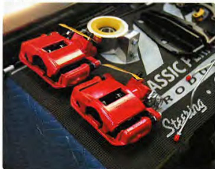
06 To complete the brakes, we installed CPP's 5-bug axle shafts, brake brackets, rotors and callipers for a killer, clean look. The custom-made calliper bracket is designed to mount directly to the backside at the axle flanges of the rear end using the provided hardware.
