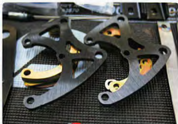
06 To complete the brakes, we installed CPP's 5-bug axle shafts, brake brackets, rotors and callipers for a killer, clean look. The custom-made calliper bracket is designed to mount directly to the backside at the axle flanges of the rear end using the provided hardware.
