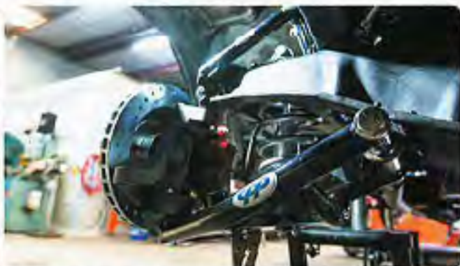
14 On this build we will be testing out Classic Performance Products all new Totally Tubular control arms and coilovers for a static yet adjustable suspension. After installing the lower control arms, upper control arms and coilovers, you can get a real feel for how well this system was designed. Fully adjustable, incredibly strong and engineered with a DIY mindset.
