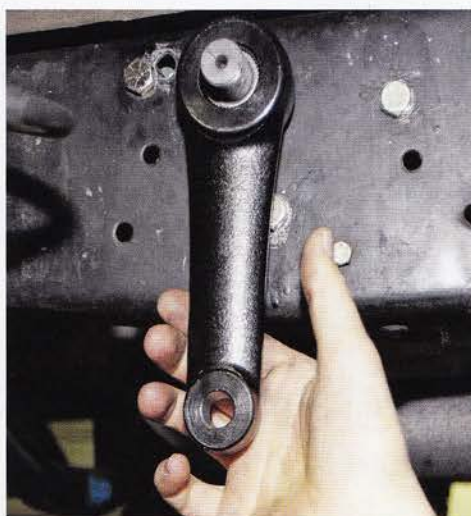
18. The new pitman arm is clocked and attached before being mated to the original drag link.
