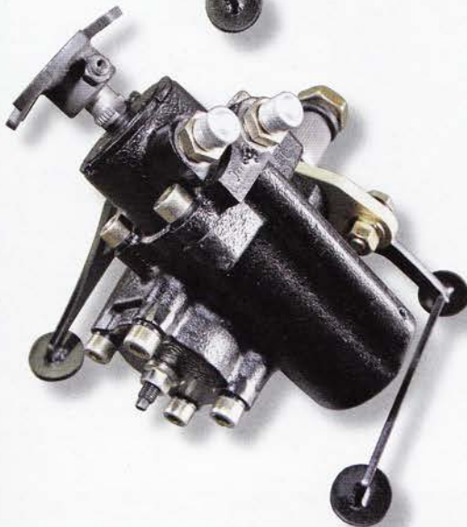
11-4. A 360-degree look at CPP's new power steering box shows a number of features that make it a great upgrade for old trucks.
