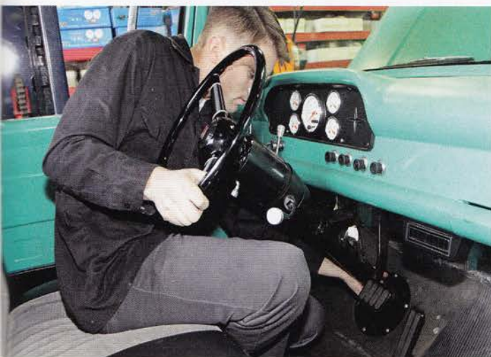
15. From there, the column can be slid into place...
