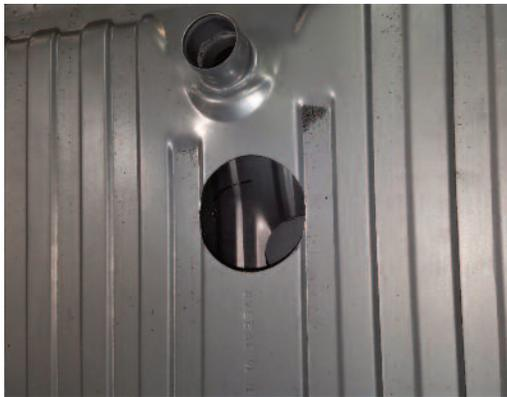
**Caution edges will be sharp once hole is cut through the fuel tank.**
