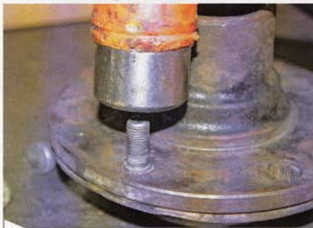
The wheel lug studs also need to come out since they are holding the inner shell on, too. Same rules apply here as with the rivet removal.
