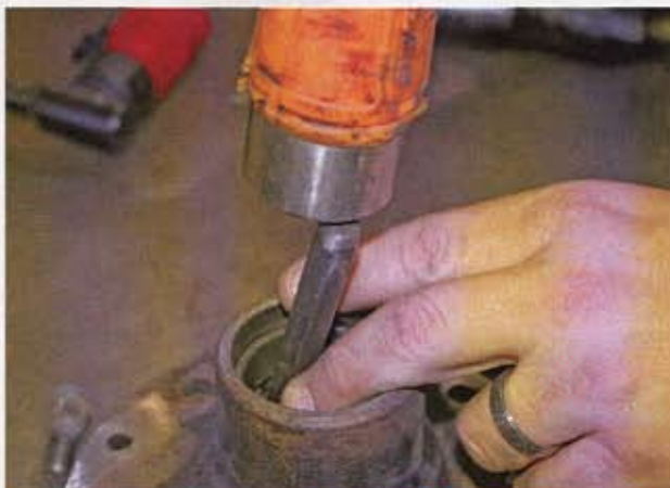
Separating the two parts reveals the backside of the hub, which will later be mated to the new disc brake rotor. We can also get a good look at the inner wheel bearing and the ancient grease seal that's made from felt. We obviously have better seals these days than the ones the big automakers used over 50 years ago, so this seal will be changed to a modern rubber lip seal (a CPP exclusive) upon reassembly.
