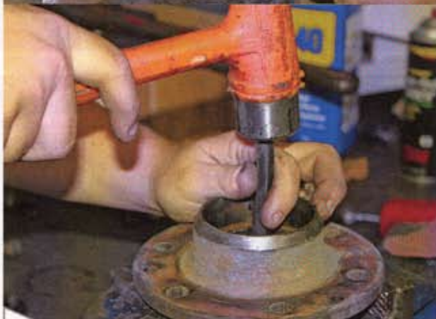
With the hub now clean and void of wheel bearings, the bearing races need to come out. I believe there are tools to do this, but most of us don't have them, so we do it the old-fashioned/precarious way—with a hammer and punch. From the backside of each race, CAREFULLY drive out the races while taping around the circumference of it as you go.
