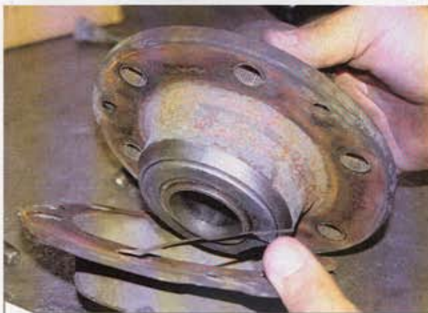
Separating the two parts reveals the backside of the hub, which will later be mated to the new disc brake rotor. We can also get a good look at the inner wheel bearing and the ancient grease seal that's made from felt. We obviously have better seals these days than the ones the big automakers used over 50 years ago, so this seal will be changed to a modern rubber lip seal (a CPP exclusive) upon reassembly.
