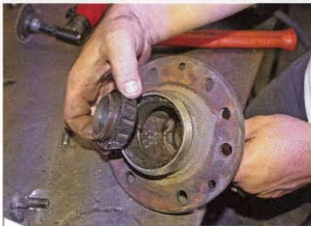
Most often, the pressed-in tin felt seal retainer will need to be pried out of the hub and is usually rendered useless in doing so. Sometimes a sharp punch driven into it at an angle is a good way to get a stubborn one out. With that out of the way, the inner wheel bearing can come out and the hub can be degreased and cleaned up.
