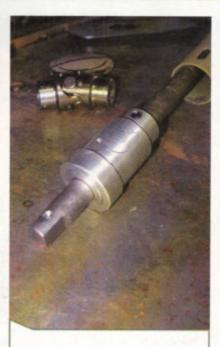
Next, the steering wheel was removed from the shaft in order for the Column Saver to be completely installed—which requires the shaft to come out from the bottom of the column.
