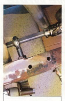
While many two-joint steering systems don't require it, if you have the room, include a support bearing on the intermediate shaft as shown. I drilled my framerail boxing plate to mount, but these are also available with integral frame brackets, too.
