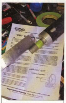
Before cutting the shaft to length, the steering wheel needs to be mounted and have around an eighth inch of play between the bell/hub and column. Having done that, I proceeded to measure and mark the shaft (notice that the lower shaft collar is in the correct location as well).
