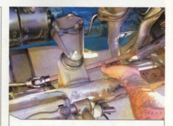
To set the correct angle and determine how much to trim the column tube back, I slipped a Flaming River 9/16-26x3/4DD joint on the rack output shaft with an oversize piece of DD intermediate shaft held in place. This also tells if there will be any interference between the rack and column, which luckily there wasn't.
