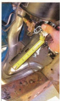
With the CPP kit, you need no less than 2 inches of steering shaft extending beyond the column tube, so I decided how far I wanted the column coming through the firewall and went from
