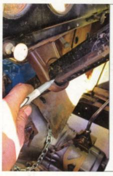
Once the column was fitted from the firewall back, the exact location of the drop was marked accordingly for future reference (and also because without proper support down below, things tended to move around without warning!).
