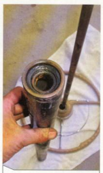
Everything was once again removed from the truck and the shaft pulled completely from the column. The upper column bearing (shown) should be replaced if necessary, or in this case, greased properly at this point, otherwise it'll affect future measurements negatively if done offer the foct. after the fact.
