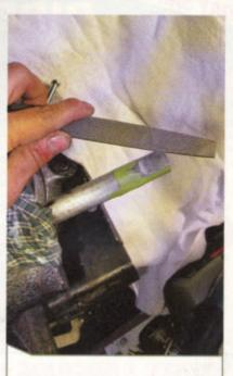
You don't need a machine shop to modify your column shaft—as long as it's not hollow, you can hand-machine it into a DD with just a couple good files and some masking tape for reference.
