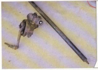
In the case of the '39, using the stock column wasn't an option due to its smaller diameter (CPP's smallest Column Saver is too big), but that wasn't an issue as I'd planned to use a '47-54 column anyway. As you can see here, first step was to sever it from the box with a chop saw.
