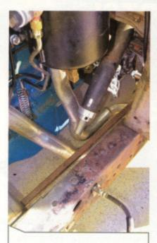
I reinstalled everything and hung them back in the truck. Using an existing slotted hole in the tube for the setscrew, the Column Saver components were loosely installed for the first time and everything checked out good so far.
