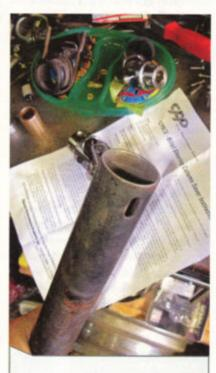
The column tube needs to be cut as squarely as possible, and once cut, make sure to deburr the opening as well as thoroughly clean the inside of the tube beyond where the Column Saver will go.
