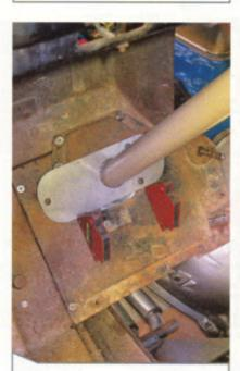
On this particular model, the stock, two-piece toeboard portion of the floor is not too accommodating to the new setup—for now, I may attempt to integrate a piece like this '47-59 filler plate from CPP. However, it's looking more like I'll be replacing the floor completely using a kit from Direct Sheetmetal instead.
