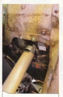
To secure the bottom of the steering column to the truck, I ended up modifying CPP's basic '47-59 column floor mount to work on the engine side of the firewall—as such, it not only kept the area clean inside, but is very inconspicuous mounted like so.
