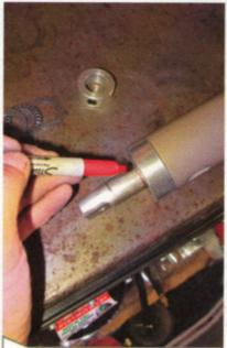
With just the billet column adapter portion inserted into the column, I marked the steering shaft right where the bottom edge of the adapter was—this will tell me where to locate the lower steering shaft collar, which will in turn dictate where the upper one goes.
