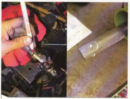
In order to allow the Flaming River U-joint setscrews to do their job, the surface to which they set should be slightly "indented." I did so after mocking things up and clocking, or phasing, the U-joints correctly so I wouldn't end up drilling extra holes.
