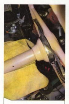
Now that the steering shaft had been cut, machined, and drilled accordingly, the steering wheel was reinstalled and the two slipped back in the column. (Here's where you could get in a little trouble if you didn't already address the upper bearing situation.)
