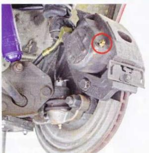
On some Mopars, the same right and left calipers "swapped sides" based on whether the installation used a leading or trailing caliper mounting position. On this front-mount (leading) install, the driver-side caliper is mistakenly mounted upside-down-the bleed screw (circle) faces down, when it should be at the top of the caliper, facing up. This unit belongs on the passenger side. No wonder the brakes wouldn't bleed!
