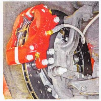
[This 1955 Chevrolet fullsize passenger car is running a Wilwood Engineering front disc-brake conversion kit. The old Chevy is a "rear-steer" car; that is, the steering box is located behind the drag link and front spindles. The calipers are front-mounted for more steering-linkage clearance.
