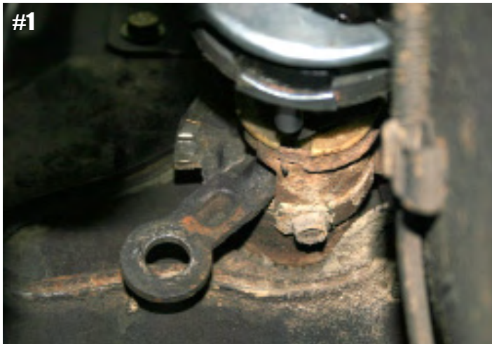
Photo #1 Again, apply the parking brake then place the steering column shifter in the Park position. Remove the stock linkage and bushing from the steering column's shifter bracket.
