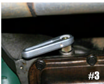
Photo #3 The aluminum arm supplied in the Shift Linkage Kit is installed next by sliding it over the corresponding splined bushing. Place the arm in the 8 o'clock position (Park). The kit contains
