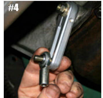
Photo #5 A complementing swivel rod end is then mounted onto the steering column's shift bracket utilizing washers and spacers. Once tight, the swivel must be free to rotate!
