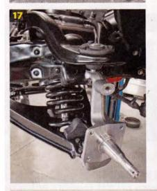
The coil won't seat properly unless it's positioned/clocked correctly in the lower spring pocket.
