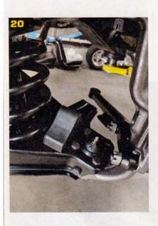
20 With the control arms "buttoned up" so to speak, the new steering arm is installed and either reconnected with the existing linkage or...
