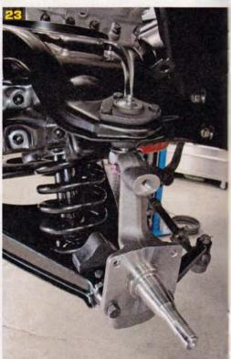
If replacing the entire assembly as such, it is probably best to disassemble the old linkage as a whole, which will allow you to assemble the new parts with similar geometry. Note the addition of CPP billet aluminum tie-rod adjusters.
