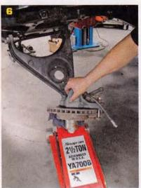
Because the coil is under extreme load, a spring compressor is securely installed with the spindle still attached. Once the coil is compressed, a floor jack is placed under the lower control arm and the upper ball joint nut is removed.
