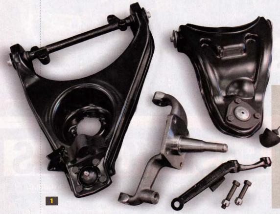
Along with complete frontend kits (tie rods, idler arms, ball joints. etc.), Classic Performance Products' OEstyle suspension parts are highlighted by their stampedsteel control arms and further complemented by original replacement spindles and steering arms.
