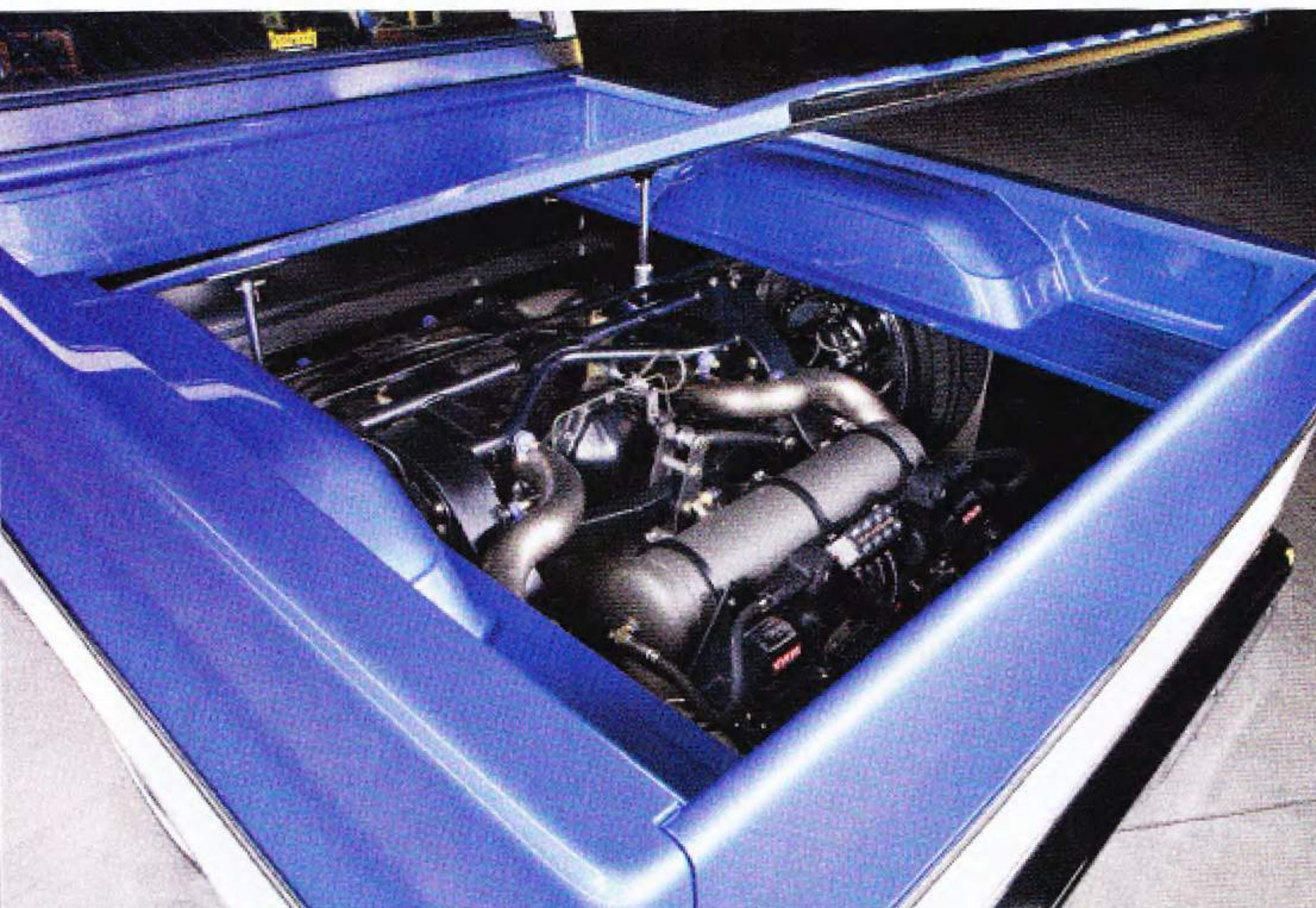
THE BED FLOOR LIFTS UP TO REVEAL THE CUSTOM SUSPENSION AND AIR MANAGEMENT SETUP UNDERNEATH.
