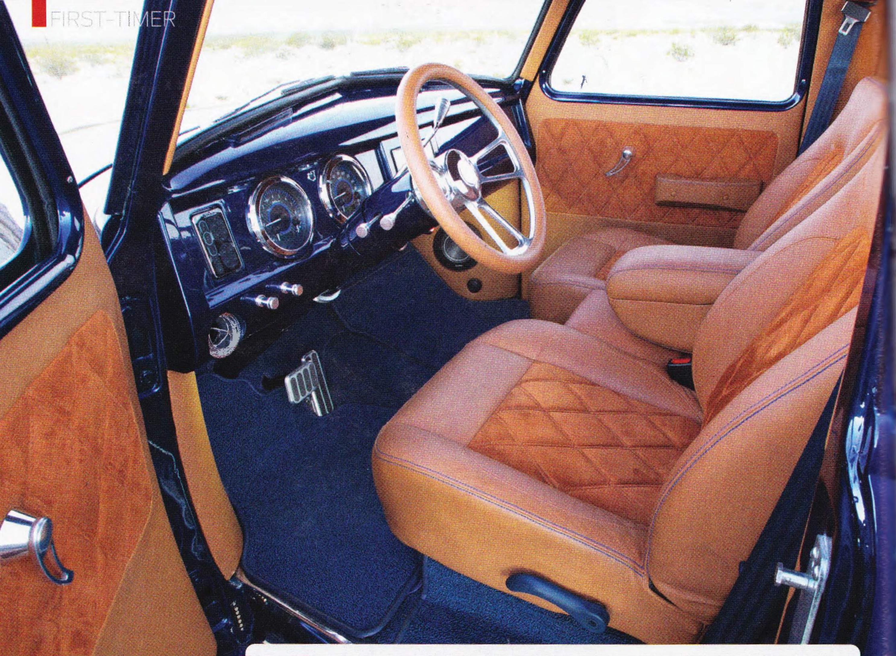
THE INTERIOR COMBINES THE OLD WITH THE NEW, USING A CUSTOM DASH AND CHEVROLET COLORADO **BUCKETS WITH DIGITAL GAUGES** FOR A TRICK LOOK.
