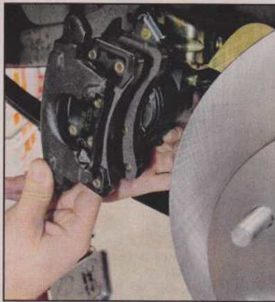
5. The calipers were mounted, with the bleed screw toward the top.
