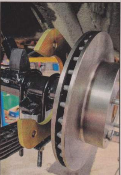
4. The rotors were now installed on the axles.
