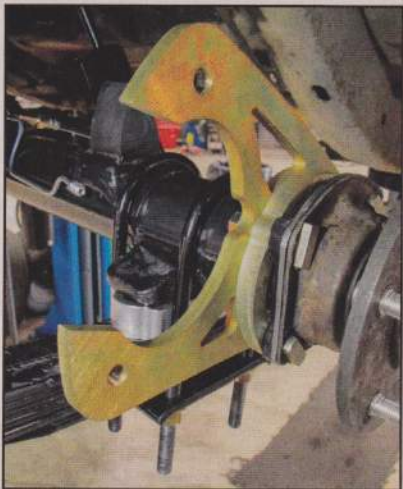
3. A spacer and the caliper bracket could now be installed, and nuts installed on the 3/8-inch bolts passing through the retainer, shim, housing flange, spacer, and bracket.
