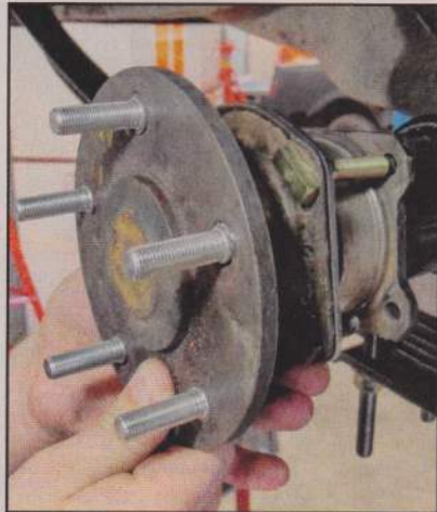
2. The axles were now installed in the housing. Note we'd also replaced the wheel studs while the axles were out.
