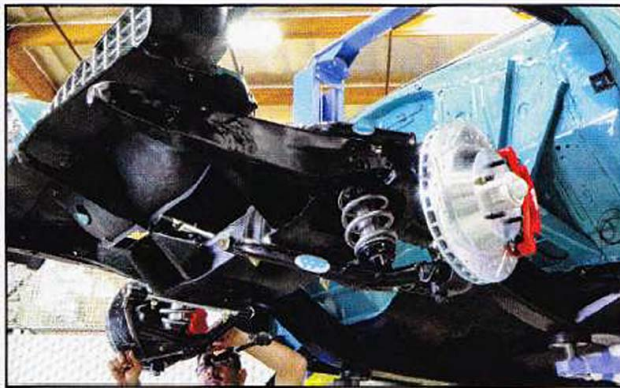
11. Again using the floor jack, the lower arms were raised until the upper ball joint could be located in the spindle.
