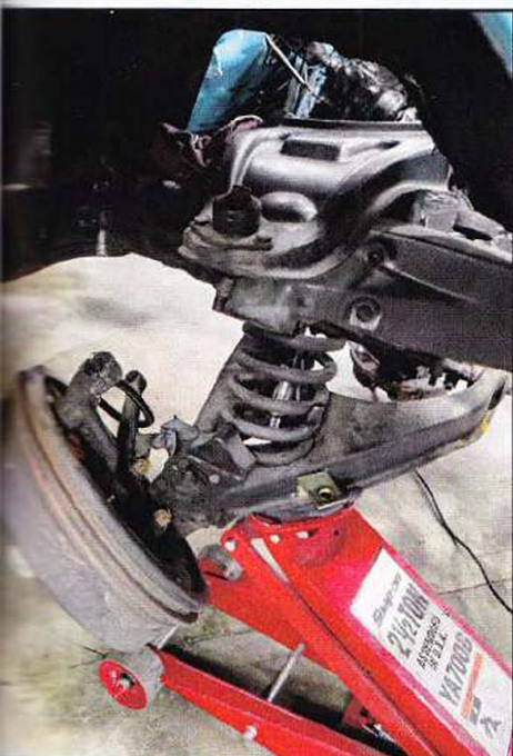
2. With a floor jack under the lower control arm, the upper ball joint was undone to release the upper arm. With the shock absorber removed, the jack was let down slowly to release tension on the coil spring. If done carefully, this negates the need for coil spring clamps. Once all tension was released, the coil could be removed, followed by the upper and lower arms.
