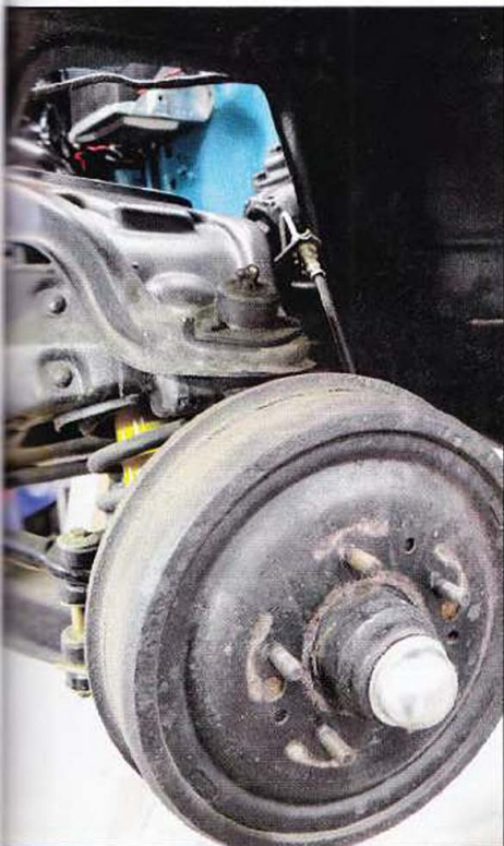
1. The stock pressed steel arms and drum brakes; not quite up to today's performance requirements, despite having been updated with a new sway bar and shocks.
