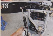
Now that the upper and lower arms and coil were in place, the CPP modular dropped spindle and big front brake kit were installed. The spindle and brake assembly is lowered onto the lower ball joint to prepare for hardware to
