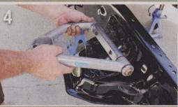
The CPP Totally Tubular upper control arm is installed onto the factory mount on the frame. The CPP arms install with ease in the factory location using all factory hardware, and they are engineered with precise geometry for paramount performance.
