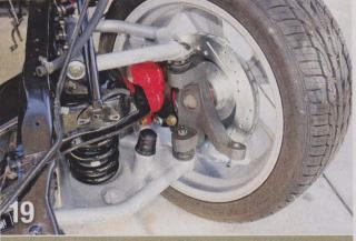
Here's a great view of the CPP front suspension. This system installed easily, using basic hand tools, a floor jack and jack stands in our driveway.
