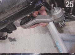
The Rare Parts pitman arm is installed onto the base of the steering box spline and tightened up. Rare Parts has all the parts you need to completely treshen up your steering.
