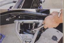
Using a socket and ratchet we made the rounds with the UCA (upper control arm) hardware to seat the CPP Totally Tubular arm into its position of performance.
