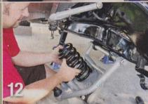
Here is the completed CPP front suspension for the C-10 with the Totally Tubular control arms, modular dropped spindles, dropped coils and CPP 13-inch big brake kit.
