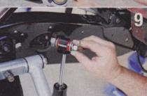
On the lower control arm there are two locating holes on the super strong 4041 billet aluminum alloy cross shafts. These are used to precisely locate the control arms in the saddles before securing the hardware and locking them down.
