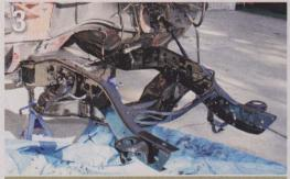
After a few hours of degreasing, cleaning and painting, our C-10 frame looked brand-new, and we were ready to hang the performance stance-enhancing suspension from CPP.
