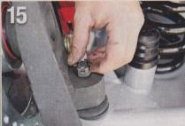
The top of the spindle and upper control arm are joined together by sliding the threaded stud of the ball joint through the top of the spindle, threading on and tightening the supplied castle nut.
