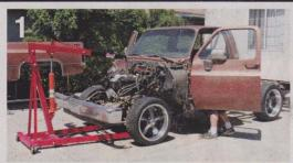
Since this truck will be getting a new drivetrain, we went ahead and removed all of the front sheet metal, pulled the bed off for a future installment where we will add the CPP trailing arm rear conversion, and pulled out the engine and transmission.
