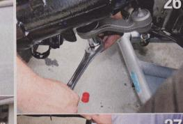
The factory center link was cleaned up, painted and reinstalled to tie the new steering parts together.
