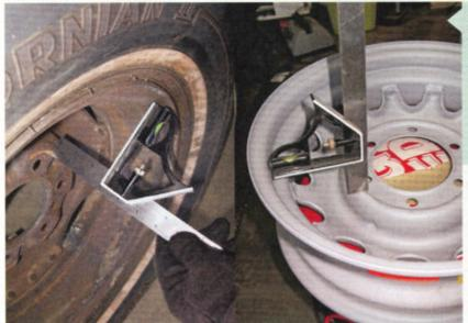
Just to be on the safe side, measure your backspacing as well as the inner diameter from the mounting surface to the outer ring (where center attaches to hoop). A majority of the early wheels have limited space behind the lug flange, whether it's large rivets or the particular "step" in the rim.
