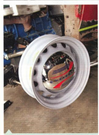
When it comes to hubcaps, you're limited to using Wheel Vintiques repops (retainer rings are different size than OE caps). The '41 passenger car style will do just fine for now-I may modify a set of originals down the road.
