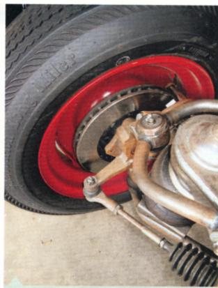
With the standard-fare 11-inch GM rotor, there's more than sufficient wheel clearance—that's due to the rotor's smaller-diameter lug surface. With a 6x5.5 pattern, you need more meat, which means a bigger rotor.
