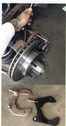
CPP's kit is designed to fit the "standard" Mustang II spindle with the perpendicular upper mount (not all MII spindles are the same!). Verify this along with inner wheel size before ordering.
