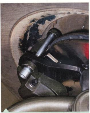
In the past, the rivets attaching the wheel center to the rim were usually the main cause of interference—but as you can see, they don't even come close to contacting anything now.
