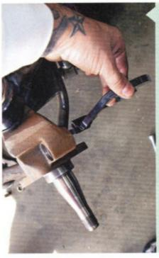
While the typical cast caliper bracket features an integral spacer on the lower mounting hole to indicate right and left, the CPP steel brackets dogleg toward the frame and do not require a spacer.
