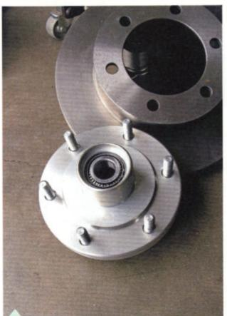
As I mentioned, the rotors are off-the-shelf Toyota Tacoma items (as are the wheel bearings), but the hubs are all CPP.
