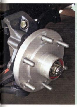
While having a twopiece rotor and hub assembly is nice when it comes to the initial install (less cumbersome not having to hold a heavy rotor), just remember that rotor doesn't stay put like it used to when you pull the wheel off.
