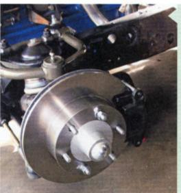
The base kit comes with a non-drilled rotor-which is more than sufficient for an old truck running a 235 engine (yet more brake than it had beforehand). For higher-performance applications, CPP can upgrade the rotors accordingly.
