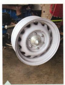
Just as I was installing the new brake kit, Wheel Vintiques came out with their steel artillery-style wheels. While they are available in 16s, I wanted to see if the 15x5 would fit.
