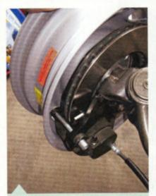
With a 2-inch backspacing, there isn't any interference between the wheel and the brakes whatsoever. Unfortunately, I can't say the same for all early GM 15-inch wheels.
