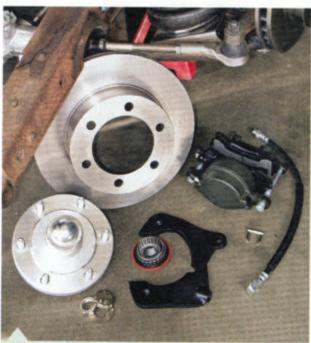
More meat is just what CPP's kit has with its 11 11/16-inch Tacoma rotors and Big Bore metric calipers—both of which fit nicely in (most) early 16-inch factory wheels.
