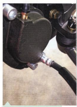
Unlike the smaller S-10 calipers, there's no right or left with the Big Bore brakes-install with the bleeder valve on "top". If you try and reuse your old brake lines, make sure the banjo fittings seat correctly, or avoid the issue and use the new ones!
