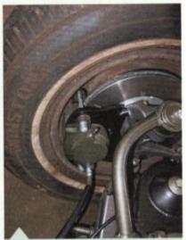
I attempted to fit a 15-inch six-lug wheel off a mid-'50s Chevy truck, but it wouldn't clear due to its offset (3-inch backspacing). A spacer would help, but at the same time you'd sacrifice available lug threads. If you're set on running a wheel as such, you'll need longer lug studs.
