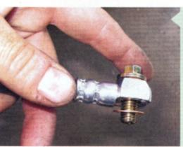
The kit comes complete with DOTapproved rubber brake hose. Along with replacing your existing ones, don't forget to install the new crush washers, too ... unless you don't mind brake fluid all over your new parts.
