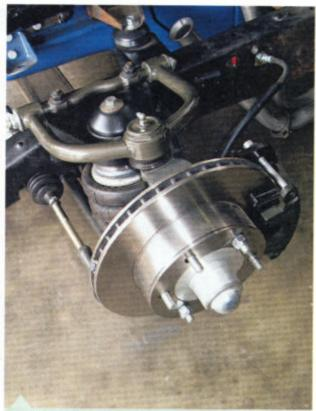
Up until now, in order to run six-lug wheels on a truck with a Mustang II frontend, you either had to shell out some serious coin to have a custom set of brakes made, or perform some questionable modifications. That's all a thing of the past thanks to CPP's new brake kit.
