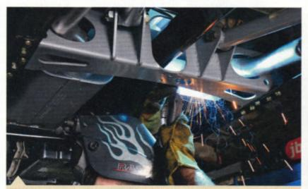
With the dump location set and everything else in place, the outlet of the muffler is welded to the rear portion of the exhaust. From the back light of the welder, you can better see how the tubes pass through the CPP trailing arm crossmember.
