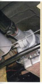
Due to the larger size of the 50 Series SUV mufflers, it was a bit of a squeeze to get them in the chassis. Their larger size will reduce noise and resonance to hopefully help me keep my foot out of the not-so-loud pedal.
