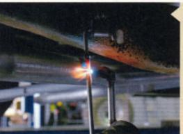
Toward the rear there was more room. A standard hanger was botted to the frame in an existing hole just above where the tube passes under the frame on its way to the front of the tire. The long rod section is heated, bent around the pipe, cut, and welded to it.
