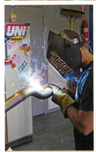
Here is the muffler side of the first head pipe and its two short and quick bends. I know it will be a bit tricky to remove the whole exhaust system when it's done (in fact it'll be real tricky once it passes through the crossmember), but at least I won't be dragging any of it!
