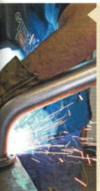
Once Josh is happy with the fit of the tubes, they are systematically welded together out of the truck before being welded to the muffler. With an installation like this where tubes pass through the chassis in confined spaces, you have to make sure you can get to the joints that need to be welded in the chassis with the welder.
