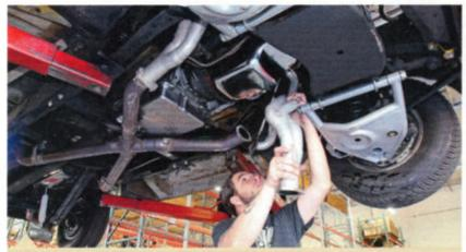
Here is the old exhaust system that was in the '72 with its X-pipe that ran under the transmission and over every speed bump and driveway in Southern California, basically destroying the exhaust after only a couple of years. This is the reason I wanted to use the Classic Performance Products' trailing arm crossmember with the holes in it to run the exhaust up in the chassis and out of harm's way.
