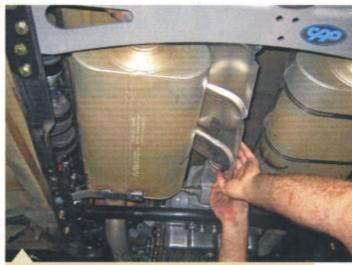
The heat shields simply fit on top of the mufflers and are held in place by these giant clamps. Put the heat shields on first if you have tight space restraints such as I (just a tip!). Flowmaster also has exhaust tips and many other accessories to go along with their U-Fit Dual Kit.
