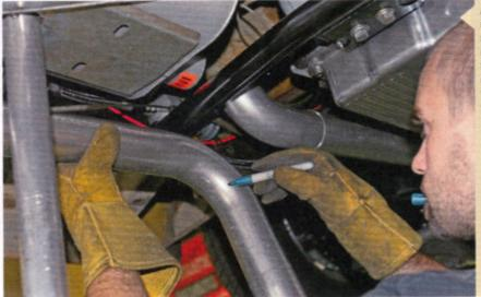
A corresponding piece of angled tube is marked and will be cut to hopefully join the muffler. Everything gets tack-welded together along the way once each piece (or pieces) fit.
