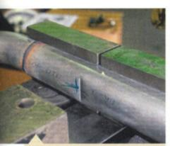
One other matter of business on the left head pipe was to clearance it just a bit for the shift linkage. Josh has a hydraulic bender that he used to dimple it, but you could do it at home with a torch, a hammer, and a large bolt or piece of rod.
