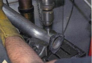
My system also needed oxygen sensors in it for the LS engine that I recently installed. Josh marked and drilled out the holes for the sensors before welding in the bungs.
