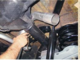
For those going over the rearend of their truck, Flowmaster includes these mandrel-bent tubes that are bent over 90 degrees that do just the trick. For really low trucks, just make sure you have enough room between the rearend and any suspension parts and the bed floor when the suspension bottoms out or altered with air bags.
