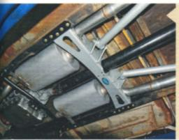
Yes it is a tight fit with the mufflers on each side of the transmission and driveshaft, but it all worked out nicely in the end. The space under the bed of trucks with trailing arms gets a bit tricky since the arms cut diagonally across what would normally be a good places for the mufflers. Those with parallel leaf springs might have more options.
