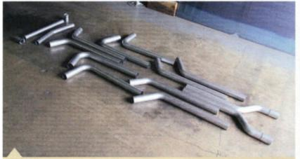
Naturally, the Flowmaster U-Fit Dual Kit comes in a big box. Once you unpack it, lay it all out on the ground in some sort of symmetrical arrangement. To help visualize it fitting under your truck. The two smaller tubes to the left are for an H or crossover pipe and the flanges to go with it, should you so choose.
