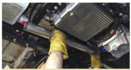
Over at the Muffler Man in Placentia, California, Josh has started with a head pipe coming off the header with a 90-degree bend in it that leads back to the inlet of the muffler. When it comes to exhaust work, you have to leave yourself plenty of leeway with the pipes until you are sure they will fit properly. See how he can't quite get the head pipe up over the trans crossmember until it is cut?
