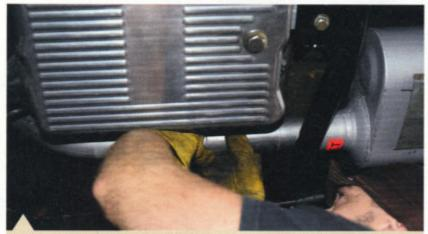
For the head pipe on the right side, a tube with a 45-degree bend in it worked where the header collector terminates. Along with this, a short length of straight tube and the connection to the inlet of the other muffler are made.
