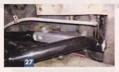
Though shown while the upper arm mounts were at the prototype stage, you can clearly see how plenty of adjustment was built in to the suspension for future alignment. It may look like a lot of shims have been used, but there's only a 1/2 inch of adjustment for camber.
