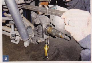
The plumb bob was also used to determine the track width, measured from the spring pocket to the inner bearing face on the spindle. This was done with the suspension under load, and shown here mocked up. The original plan was to reuse the stock wheels, but the 5-on-5 bolt pattern (to match the hubs and rotors already fitted) dictated otherwise once the Chevelle hubs were installed. However, new wheels of the same offset were used.
