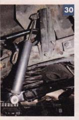
The tube shocks and antiroll bar brackets were re-attached to the lower arms, the shock mounting to the same towers that had previously been added (the original shocks would have been integral to the knee-action upper arms).
