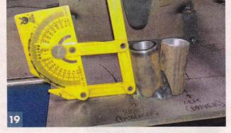
The same jig was used for the opposite arm, though the angle of the ball joint had to be copied and flipped right to left.
