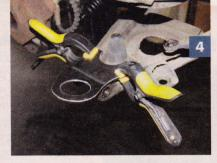
A new lower ball joint mount was mocked in position to determine everything would fit. This placed the ball joint forward of the stock lower kingpin joint as required.
