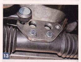
This plate was also made as a starting point to determine where the inner tie-rod ends should mount to the steering rack.
