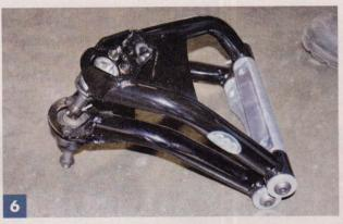
CPP provided a pair of '64-72 Chevelle upper control arms (top) as well as a pair of '55 Chevy arms (bottom), so we could determine which would work best for the conversion. Points to consider were the placement and angle of the ball joint, as well as the latter having the correct taper to match the Chevelle spindles. At this point too, Davies was trying to make the job simpler by mounting the upper arms to the stock knee-action upper arm mounts.
