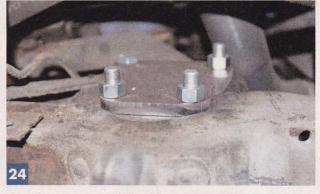
These plates were made to bolt to the original upper arm mounts ...
