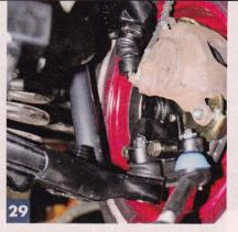
Here's a better view of the dropped spindle and the modified, boxed, lower control arm.
