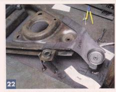
Here's how the ball joint cup was attached to the control arm, substantially stronger than the temporary method it replaced.
