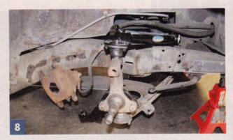
A couple of things are going on in this picture. First, Davies was experimenting with the placement of the upper control arm mount using the '55 Chevy arms. Secondly, he was trying a '67-69 Camaro steering arm. The idea behind this was that it was from a rear-steer car, so the Ackerman would likely be close to what was required, but it had way too much drop, and placed the tie-rod end in the wrong place in relation to the steering rack.
