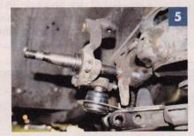
With the ball joint mount tacked in place, a pair of junkyard Chevelle spindles was used for setup purposes. Davies then began experimenting with steering arms.
