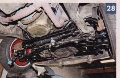
Though the tie rods have yet to be connected to the steering rack, '67-69 Camaro tie rod adjustment sleeves were used in the final version, and you can see that CPP dropped Chevelle spindles have replaced the stock versions now. The new wheels have the same backspacing as the previous ones, and as the suspension was designed with the same track width, we know they'll have sufficient clearance.
