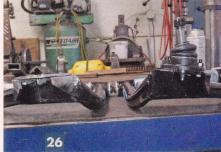
While the Chevelle upper arms eventually worked out to be the best fit for this application, there was still a small amount of bind in the ball joints, owing to the angle of the arm. Davies modified the arm as shown on the left to cure this.
