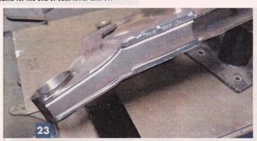
Upper and lower plates were TIG-welded in place before boxing plates were added.
