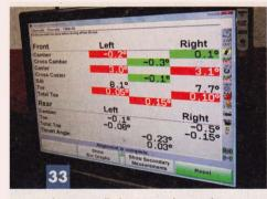
The screen tells the story; with some shims removed from the upper arms, the camber is about as close to 0 as it could be. Each side has 3 degrees of caster, and the total toe is 0.15 degree.
