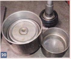
A pair of ball joint cups were machined on the lathe for the end of each lower arm ...
