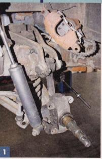
Here's the stock Olds suspension, though someone had previously added tube shocks, a steering rack with dubious geometry, and disc brakes. While adequate for highway speeds in the '50s, this setup had negative caster, and the car would change lanes at freeway speeds.
