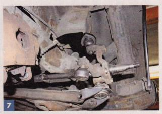
Chevelle spindles were selected because the measurement between the ball joints was as close as possible to the distance between the stock kingpin pivots. Also, they accept bolt-on steering arms, which makes them ideal for front- or rear-steer applications (meaning whether the steering rack is behind or in front of the spindle). Here the steering tie rod is being mocked up.
