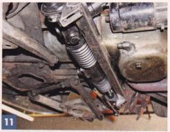
The rack in position. Note how it clears the oil pan and starter of the 455 engine.
