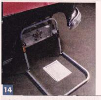
With the steering mocked up, a bumpsteer gauge was connected and the suspension moved through its travel. This showed the steering arms were way too long, so the central bracket was made longer to bring the inner tie rod pivot outward.
