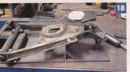
With the steering geometry set, the lower control arms could be finished. A jig was fabricated around the modified arm.
