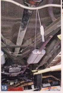
The Ackerman needed to be set before any further work could be done on the steering. With a length of string pulled taut between the lower ball joint center and the center of the rearend, the outer tie rod pivot on the steering arm should intersect the string line ...
