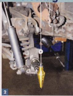
A plumb bob was hung from the front fender to determine where the centerline of the spindle was. The modifications will include moving the upper ball joint back and the lower forward when the CPP Chevelle spindles are installed, to correct the caster geometry, so establishing this baseline is important.
