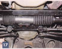
Slightly out of sequence as it's all painted, this is what the final steering rack center bracket looks like. With this bracket, the bumpsteer gauge read a total of 0.150 inch of deflection throughout the travel, compared to 2 1/2 inches with the first bracket, and the Ackerman yet to be set. The steering is turned here; the tie rods are not offset!
