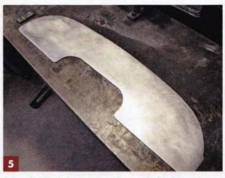
A piece of 3/16-inch aluminum plate will serve as the foundation and structural support for all our underdash needs — brake pedal/master, fuse panels, master kill switch, even the battery.
