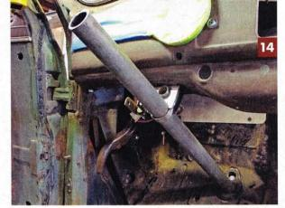
And to properly locate the brake pedal, we mocked up a dummy steering column using a piece of 1 1/2-inch exhaust tubing, as so.
