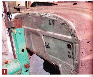
What's a true custom without a shaved 'n' smoothed firewall? Well, for one, it's an area void of allowing any type of through-metal attaching for components beyond its exterior surface—like a wiring panel, or in our case, a brake master cylinder/pedal assembly. Another case of form before function? Let's see if we can remedy that.
