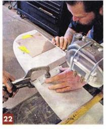
Once that was done, the holes for the brackets were marked and transferred onto the plate for subsequent drilling and tapping.
