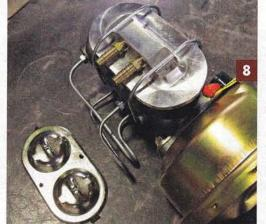
As mentioned, we wanted to retain as much space behind the dash as possible for future access reasons — including having to check/fill the master cylinder. That said, however, we're also considering a remote-fill option using CPP's billet-aluminum reservoir lid, tapped for ports allowing fluid to be serviced elsewhere (as long as it's from a higher vantage point, which is our main obstacle at the moment).
