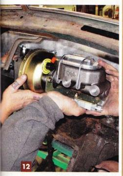
In case we're unable to enable a remote fill setup, we wanted to see just how close the master cylinder reservoir was to the cowl vent, as that may be a viable option for future access. Of course, one major drawback to that: potential fluid spillage, something a nice paintjob will not accept!
