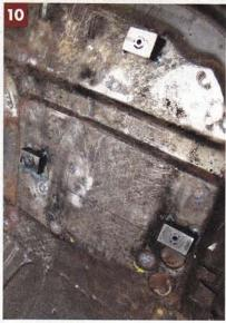
With the firewall plate shaped with its mounting tabs attached via countersunk Allens, the panel is final fitted and points marked where the tabs will be welded onto the car.
