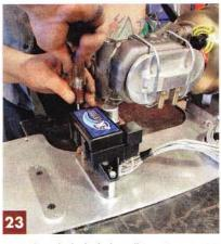
Here's how she looked when all (most) was said and done. Notice we rotated the boxes 45 degrees in order to route the wire looms horizontally along the panel, eliminating having to loop them up and around.
