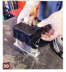
Knowing this also led us to come up with a pedestal-type bracket in which to mount the panels—the flat tabs attach to the firewall plate and are tapped to accept the fuse/relay panels via tube standoffs.
