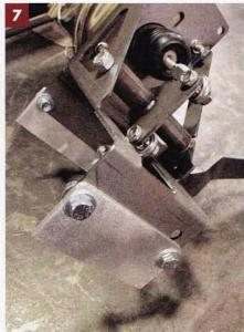
Since the CPP booster/MC bracket is steel, JBC fashions aluminum tabs that weld to the firewall panel. Gussets will be added to further strengthen the mount, helping avoid any structural failure once the brake system is put to use.
