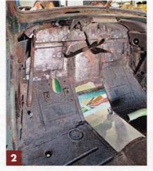
Sure, welding studs/captured nuts to the interior of the firewall would easily facilitate the mounting of our fuse and relay panels — but for anything of substantial weight, we need to incorporate a substantial device to support not only the weight, but the stress caused by regular use of ...
