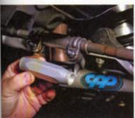
Besides the lighter weight of CPP's aluminum sleeves, there is some added practical utility. The stock sleeves are stamped from steel, and leave crevices for water and road dirt to accumulate. Over the years, rust can develop, causing the clamp nuts to freeze in place.
