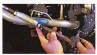
Thread the adjuster sleeve onto the inner and outer tie-rod ends after you have threaded the locking jam nuts on. Make sure you turn both ends the same number of times, comparing the overall length to the measurements you took earlier. When you get them the right length, tighten the jam nuts.
