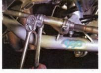
outer end links were replaced last year, but we've included the CPP part numbers in our chart. Note that the '64-70 tie rods are all the same, but the '71-72 tie-rod end links have different threading.
