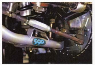
With the tie rod lengths set to your old specs and the end-links reattached to the spindles, you should be able to drive to the
