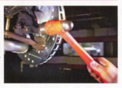
rod ends. Use a mallet to loosen the tie-rod end from the spindle (after removing the cotter pin and castellated nut). Use a pickle fork at your peril: it will usually ruin everything it touches.
