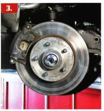
**3-5.** Disassembly of your front brake and spindle package will require your old brakes, spindles, and separation of tie-rod end related to steering.
