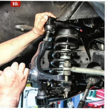
8-9. Working on the upper control arm here we are loosening the ball joint. Hand tools will get this job done—and a good hammer!
