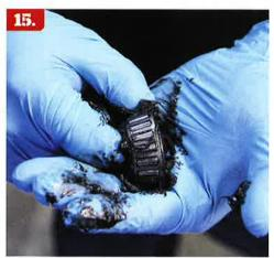
15-16. Should you purchase the complete CPP kit the wheel bearings come prepacked but should they be "dry" the bearing will need to be packed with wheel bearing grease. This can be done the old fashion way by hand (which I'm sure all of us have done at some time) or you can purchase an inexpensive and nifty wheel bearing grease tool such as the Harbor Freight universal bearing packer (PN LNL145).
