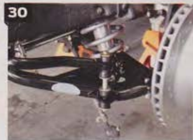
28-30. Next, slide the frame mount U-bolts through the top of the frame that holds the frame mount in place. Finally, configure the sway-bar stems on each side that attaches the bar to the lower A-arms to control the lateral forces while under load or at speed.
