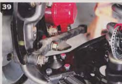
35-36. To finish off the look of the 500 series box, remove the fastener that holds down the adjuster plate, and replace them with CPP's plate cover and stainless fasteners. This gives the box a noticeably finished look.
