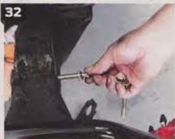
32-34. It simply goes right back into the factory location using the supplied fasteners that mount through the frame. However, you'll need to change out the factory steering column to a joint-style column that's also available from CPP.
