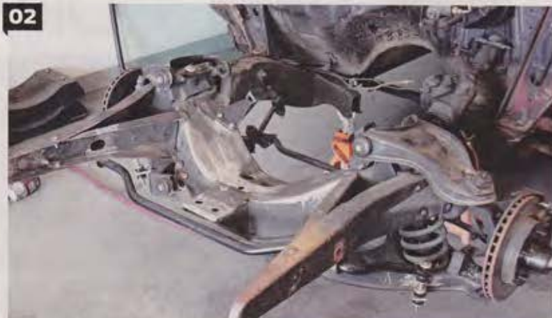
02. Because this '56 Chevy Bel Air hardtop will receive an LS swap, we removed the engine and front sheet metal. If you plan to do the work yourself, it isn't necessary to remove all of these parts. You should be able to convert everything to the new kit in one day.
