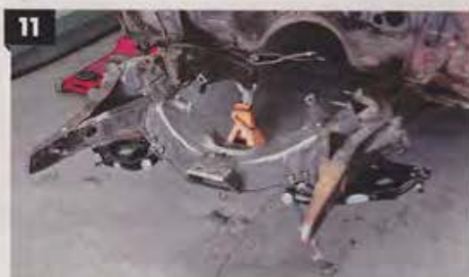
09-11. Reconstruction begins at the bottom, because the lower A-arms go in first. CPP designed the cross-shafts on the arms to bolt back into the factory arm positions. The company supplies new zinc-plated fasteners to hold everything down snugly.
