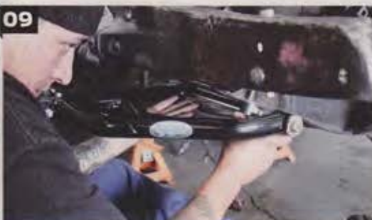
09-11. Reconstruction begins at the bottom, because the lower A-arms go in first. CPP designed the cross-shafts on the arms to bolt back into the factory arm positions. The company supplies new zinc-plated fasteners to hold everything down snugly.
