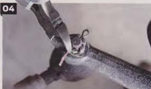
03-04. The installation begins by supporting the frame on jack stands and removing the front wheels. Next, place a jack underneath the lower A-arm at the ball joint; this will safely support the suspension while you remove the fasteners that hold the suspension components in place. Remember that the coil springs are under tension, so pay attention while removing the old components, and use the jack to slowly lower these components to avoid injury.
