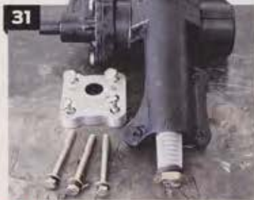
31. Upgrading the factory-style steering box to CPP's 500 series box is a must for the driver who yearns for excitement. The close ratio 14:1 produces excellent road feel, giving the driver more confidence.
