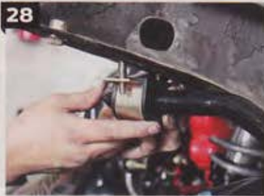
28-30. Next, slide the frame mount U-bolts through the top of the frame that holds the frame mount in place. Finally, configure the sway-bar stems on each side that attaches the bar to the lower A-arms to control the lateral forces while under load or at speed.
