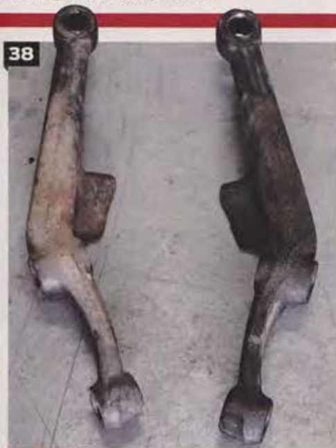
38-40. Remember back when we said to keep the factory parts? Well, we hope you did, because the OEM steering arms will marry the spindles to the tie rods. They bolt back in place using the new fasteners that come with the spindle kit. Attach the tie rods back to the steering arms and get ready to align the steering back to spec.
