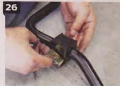
24-26. We prepped it for installation by adding a dab of urethane grease to the bushing before sliding it around the bar and securing it in place with the frame bushing band on both sides of the bar.
