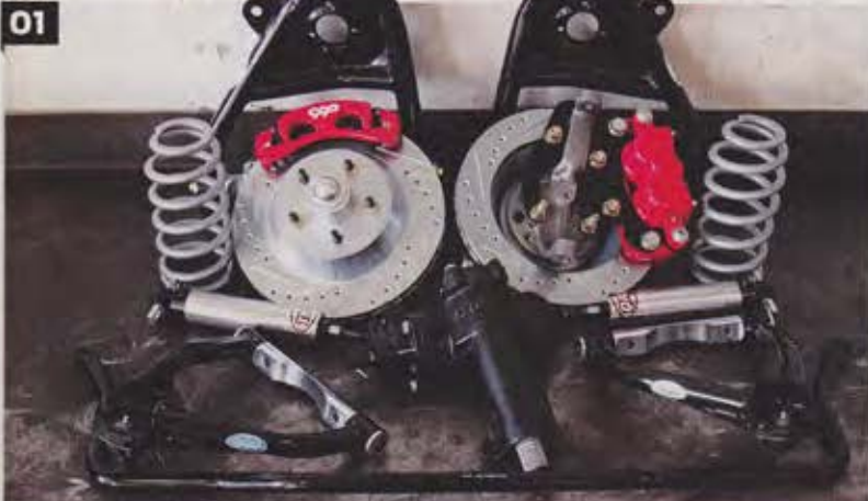
01. Included with the kit are the following parts: upper and lower A-arms, spindles, rotors and callipers, coil-over shocks, anti-sway bar and CPP's 500 series steering box.
