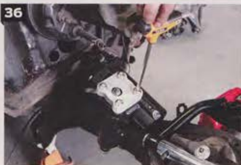
35-36. To finish off the look of the 500 series box, remove the fastener that holds down the adjuster plate, and replace them with CPP's plate cover and stainless fasteners. This gives the box a noticeably finished look.
