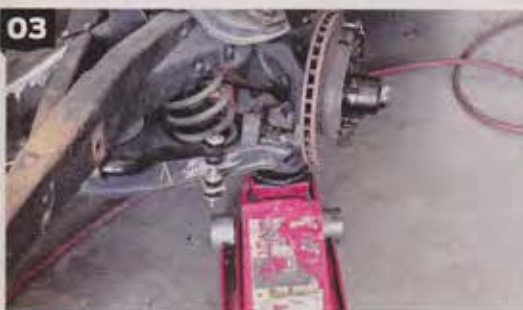
03-04. The installation begins by supporting the frame on jack stands and removing the front wheels. Next, place a jack underneath the lower A-arm at the ball joint; this will safely support the suspension while you remove the fasteners that hold the suspension components in place. Remember that the coil springs are under tension, so pay attention while removing the old components, and use the jack to slowly lower these components to avoid injury.
