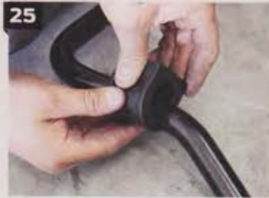
24-26. We prepped it for installation by adding a dab of urethane grease to the bushing before sliding it around the bar and securing it in place with the frame bushing band on both sides of the bar.
