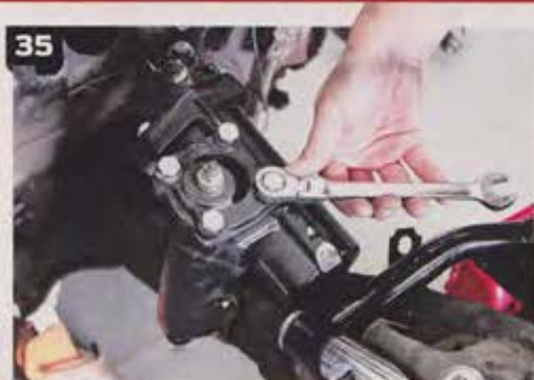
35-36. To finish off the look of the 500 series box, remove the fastener that holds down the adjuster plate, and replace them with CPP's plate cover and stainless fasteners. This gives the box a noticeably finished look.
