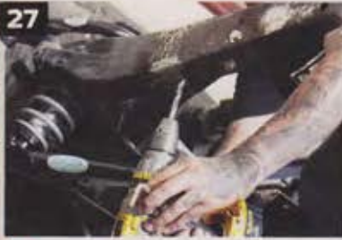
27. Using one of the factory anti-sway bar mount holes for reference, measure and drill out a new hole to accept the larger pattern where the frame-bushing band can be mounted.
