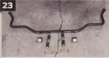
23. The official term for the next component is an anti-sway bar; however, most just shorten the name to sway bar. Its purpose is to control body roll and high-speed sway while driving. There's a fine line on how big the bar can be without creating an uncomfortably stiff ride. CPP has developed just the right-size bar that allows the best of both worlds.
