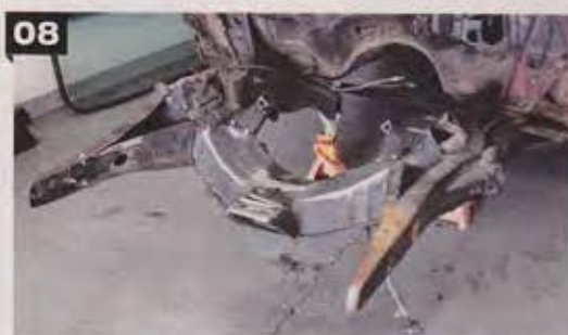
8. This is what the front end should look like once all of the components are removed.
