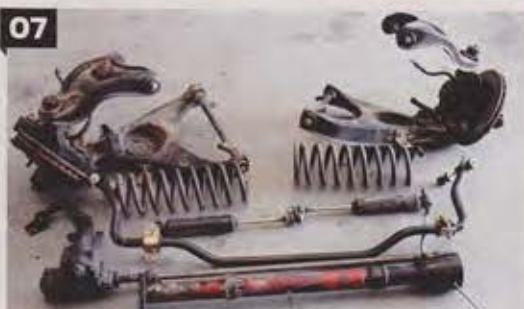
07. You'll need to drop the factory steering column and snake the column rod and factory box out of the engine bay. This can also be tricky when the engine is in place, but it can be done by removing the pitman arm before removing the box and column.
