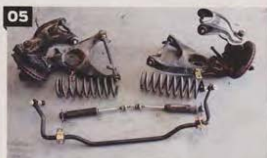
5. Once you remove the upper and lower A-arms, springs, shocks and anti-sway bar, you're halfway finished installing the kit. Be sure to hold on to your parts until the conversion is finished, because you'll need to reuse the factory steering arms on the new CPP spindles.
