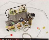
To finish the front disc brake conversion we started in last month's issue, we installed a new master cylinder, proportioning block, and brake lines, all included with the Classic Performance Products (CPP) kit. This is the most complete disc brake conversion kit we've ever installed, not requiring a single additional part, fitting, or adapter.
