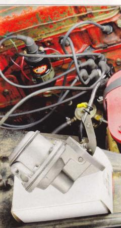
When we cranked over the engine with the ignition system repaired and upgraded, we quickly realized that the ancient fuel pump was leaking far more fuel than it was pumping. AutoZone was able to get an exact replacement within a day. The new pump even had the correct-size port fittings so we didn't have to modify the fuel lines.
