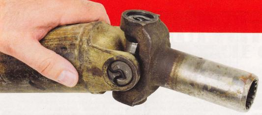
The driveshaft had been removed from the car, perhaps when it was flattowed back to the previous owner's house on the day it quit running. We had the shaft balanced and new U-joints installed in both ends. This is a good idea with any car that has been sitting, especially if the driveshaft has been removed.
