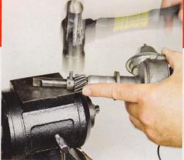
With the brakes done, we returned to the engine to figure out why the car was parked in the first place. It didn't take much detective work to notice that the distributor wasn't spinning when the engine was cranked. We pulled the distributor out and found that the roll pin that was supposed to hold the drive gear on the distributor shaft was sheared. We replaced the \$1.10 pin with high hopes that this was the only problem.
