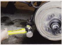
To separate the tie-rod end from the steering arm, remove the castle nut and hit the side of the steering arm with a heavy hammer. You don't need to hit it too hard, but you'll probably need to hit it several times. The impact releases the pressure on the tapered part of the tie-rod end, letting it drop out.
