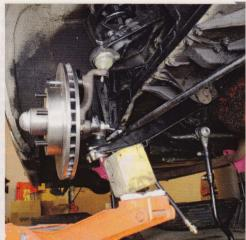
We set the CPP steering knuckle and brake assembly on the ball joint in the lower control arm first. Then we used a floor jack to raise the arm and assembly to meet the upper control arm.
