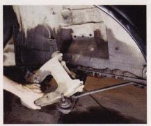
To replace the bushings in the upper and lower control arms, the arms must be removed from the car. With the spring and shock out, the upper arm unbolts from the shock tower. The lower control arm is held in place with a single bolt and a suspension alignment cam plate.
