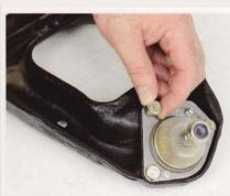
Grade 8 hardware and Nylock nuts are included with the ball joints. CPP uses Nylock nuts for the ball joints instead of a traditional castle nut and cotter pin.
