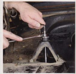
Now you can cut the nylon strap off the gas-charged shock. Install the lower washer and rubber bushing, and then guide the threaded end of the shock through the top of the shock tower. The CPP shocks for this application have an Allen fitting in the top of the shock that you can use to hold the shock rod while tightening the nut.
