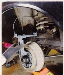
Since we are changing wheels and tires, we used a Percy's High Performance Wheelrite from Taylor Cable Products to determine the tire size and backspacing. The Wheelrite is adjustable and can simulate a variety of wheel and tire sizes, making it easy to see what will fit. The CPP disc brake kit we're using does not widen the track width—important to know if you're measuring using your old brake system like we are here. Use a jack under the lower A-arm to compress the suspension to ride height.
