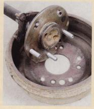
We took our axleshafts and brake drums to a local machine shop to have a five-lug pattern drilled in them. Because of the spacing, two of the holes will overlap, which is not good for strength. The new wheel studs pulled into the thick axle flange straight and solid, so we feel OK running this with our stock 140hp I-6, but we wouldn't advise this for a V-8 car.
