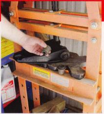
CPP offers both replacement-style rubber bushings and its Polyplus front-end kit that includes graphite-impregnated bushings for better handling and longer life. The complete kits include upper and lower ball joints, inner and outer tie-rod ends, adjusting sleeves, an idler arm, control arm bushings, and strut rod bushings. You'll need a press like this one from Harbor Freight Tools to push the old bushings out of the control arms and to install the new ones.
