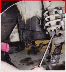
Next, the spring and shock are removed. The Chevy II has a suspension design unique in the GM family of cars, although it is similar to Ford suspension systems from the same era. It uses a spring mount on too of the upper A-arm. The lower arm is simply a straight channel with a support rod that triangulates it to the front of the car. The support rod uses large rubber bushings that we also replaced with new ones from CPP.
