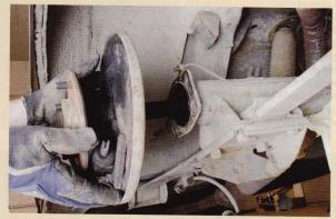
There is no easy, inexpensive, or good way to convert the rear of a '62-'63 Chevy II to five lugs. The brake drum is unique, as is the rear axle tube flange, preventing you from bolting on aftermarket brake alternatives. The only upside is that it's not a C-clip axle assembly, so you can unbolt the backing plates and remove the axleshafts to have them redrilled.
