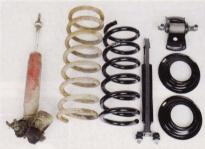
We ordered new springs, shocks, shock mounts, and coil spring plates from CPP. The company offers stock height and lowering coil springs. We opted to lower the car approximately 2 inches while we were making these changes. The new spring has the same wire diameter but is shorter, which should retain a very good ride quality.
