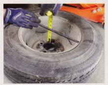
If you're not using a Wheelrite, you can measure your existing wheels and tires and measure the available space around the package when it's installed on the car. To determine backspacing, place a straight edge across the inside wheel lip and measure the distance to the wheel mounting flange. If your car has decent-sized tires on it, you can just order replacements. Our Chevy II had undersized tires in addition to having stock 13-inch wheels, both situations we'll remedy thanks to Coker Tire.
