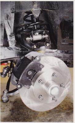
Here's the completely rebuilt front suspension and disc brake upgrade. The suspension rebuild is a critical safety step before putting a barn find back on the road, and the disc brakes will make this car stop better time after time, making the car significantly safer. We still need to install the new dual-reservoir master cylinder, proportioning valve, and brake lines included with the CPP disc brake swap kit.
