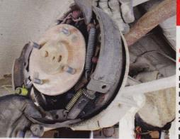
At the rear of the car, you can retain drum brakes because 70 percent of the stopping power is provided by the front brakes. We replaced the shoes, hardware, and wheel cylinders on the rear. The shoes had plenty of material left on them, but 20-year-old shoes have a way of coming apart when they are put back into service. MCR
