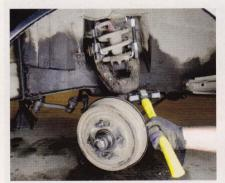
This same technique is used to release the ball joints with one important difference. We've used spring compressors to remove the spring pressure from the A-arm. On this style of suspension, you have to do this to separate the ball joint from the steering knuckle. On systems with the spring mounted between the two A-arms, the force of the spring can be very dangerous if the ball joint releases and the spring is not contained.
