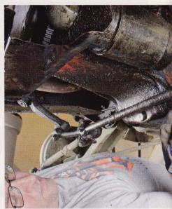
Separating the inner tie rods from the center link is a bit more challenging than freeing the outer tie-rod ends. Harbor makes a five-piece front-end service tool set that has all of the tools you need for this task as well as for removing the pitman and idler arms.
