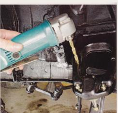
We also needed to open up the holes for the new lower spring and shock mounts in the upper control arm. This would be easier to do off the car, but we didn't mock it up for fitment until after we had the upper control arm reinstalled.
