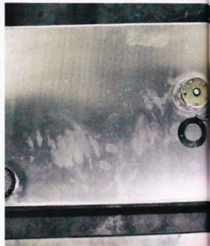
CPP's fuel sending unit can be shortened to adapt to any size or depth fuel tank. Once shortened, Luis from "House of Pain" Customs was able to mount down the unit. The Aeromotive fuel system and filter were also installed easily as per instructions.
