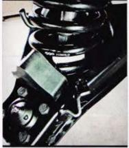
The coil won't seat properly unless it's positioned/clocked correctly in the lower spring pocket.
