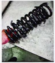
Even though we're installing a 1/2inch lowered coil, the spring still needs to be compressed for both safety and ease of installation.
