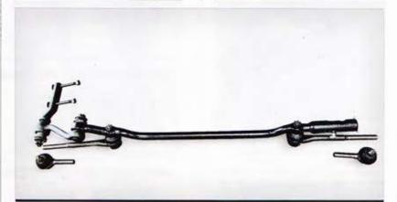
**21.** ... the job continues with the assembly of a new drag/centerlink and complete frontend kit (which includes all-new tie rods, idler arm, adjuster sleeves, and related hardware).
