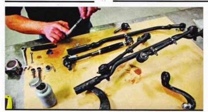
22. If replacing the entire assembly as such, it is probably best to disassemble the old linkage as a whole, which will allow you to assemble the new parts with similar geometry. Note the addition of CPP billet aluminum tie-rod adjusters.
