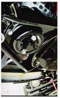
Once the ball joint nuts are securely fastened and cotter-pinned, new Black Magic nitrogen gas shocks are installed.
