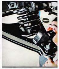
14. Compressing a dropped spring may eliminate the need to use a floor jack to button up the spindle to the upper control arm—but if any resistance is experienced, don't risk it.
