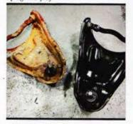
Additionally, CPP's upper control arms have 5 degrees of caster built in, not added—a for sure "plus" for power steering-equipped Tri-Fives. This will improve your lowrider driving experience with upgraded geometry.
