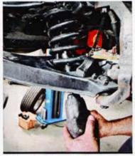
5. Since the coil is under extreme load, a spring compressor is securely installed with the spindle still attached. Once the coil is compressed, a floor jack is placed under the lower control arm and the upper ball joint nut is removed.
