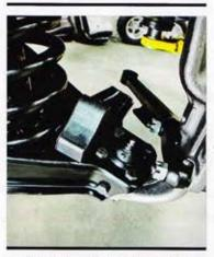
20. With the control arms "buttoned up," so to speak, the new steering arm is installed and either reconnected with the existing linkage or ...
