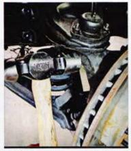
4. We started off by removing the stock '57 front suspension already equipped with a standard-type disc brake kit. First, with the ball joints' nuts loosened up ("not" removed), the spindles are given a few good whacks with a heavy hammer to help ease separation—no pickle forks used in this process.
