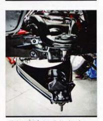
12. Control arms installed and ready to be mated with new coils, spindles, and steering linkage. As you can see, adapting hydraulic cylinders and/or airbags with an outboard shock would be simple to do. Note the orientation of the upper control arm by the location of the ball joint in relation to the lower one—if it appears further forward, you've got the sides swapped.
