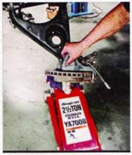
Very carefully, after the upper control arm is set free, tension on the jack is released and the collapsed coil spring is safely removed.
