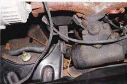
Here we have the original Steering Box.
