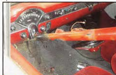
Removing the old stock column.
