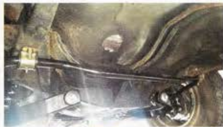
Column mounted to the firewall along with the clamp in place.
