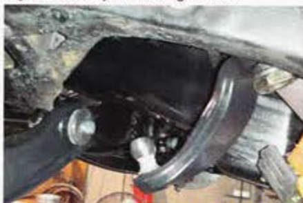
Pitman arm attached to the Power Steering Box
