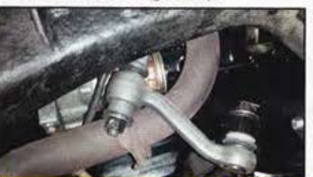
Close up of the new 505 CPP Power Steering Box with the rag joint connector.
