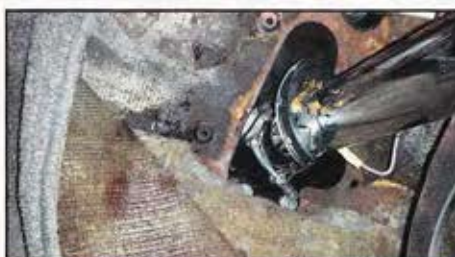
Column mounted to the firewall along with the clamp in place.
