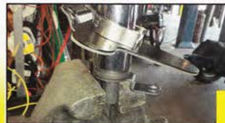
Column showing the gear shift lever firewall mounting plate and clamp.
