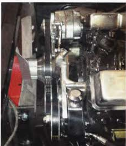
Side view of the Power Steering Pump installed with hoses and belt.
