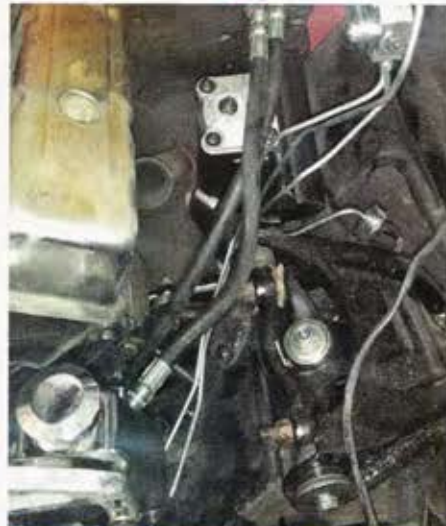
Routing the hoses away from heat, friction areas etc.
