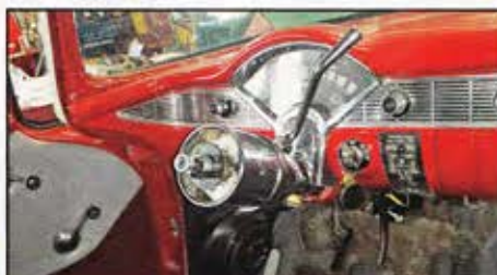
Column mounted in place with gear selector installed. Now we need to install our custom steering wheel.
