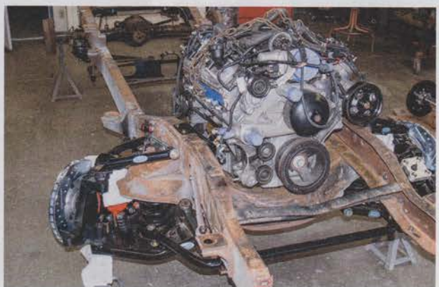
23 The LS engine fits like a glove with the GTO pan hugging the crossmember just right. The stock A/C compressor will be replaced with a smaller Sanden SD-7 unit and the top framerrails will be trimmed where necessary for extra clearance of the accessories. Even with the GTO front accessory drive, the alternator ended up clearing just fine with a small trim to the top of the framerrail.
