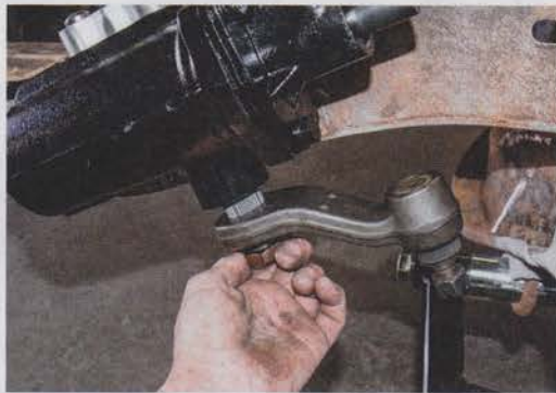
14 A new Pitman arm is installed on the new box before the centerlink assembly is attached.
