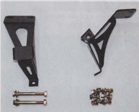
16 CPP's engine mount stands offer plenty of header clearance and are a stark contradiction to what was previously available for these old trucks.
