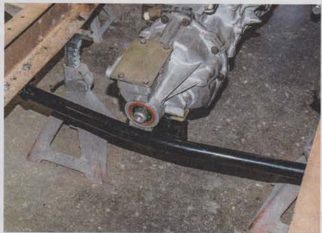
21 With the motor resting on the mounts at the front, the transmission crossmember can be located. Once in place, it's checked for center and then the holes can be drilled in the chassis and the assembly mounted for good.
