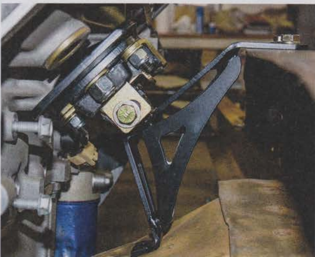
22 With the motor in place, here's a look at the assembled engine mount.
