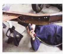
**12-15** Once the forward bracket is bolted in place, you will need to drill an additional hole on the underside for a sixth Allen bolt to go nearest the rearend.
