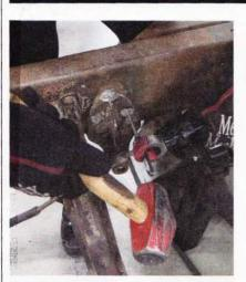
**07-08** Of the many methods in which to remove rivets, we've found the following procedure to work very well: grind exterior rivet head flush; center-punch and drill rivet through frame, but not entirely through backside (leaving remaining head fully intact); hammer out using a drift slightly smaller than rivet body.
