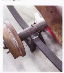
18-19 The rearend was set atop jackstands (with the pinion supported via the floor jack), the new spring pads were set in place, and the leaves shackled up in the rear, as such. (Notice by the evidence left by the old U-bolts how far off the original leaf springs potentially were.)
