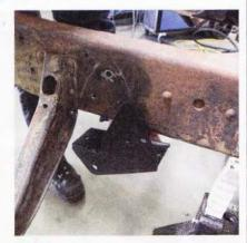
10-11 As mentioned, the new fabricated brackets locate off the existing holes. On the forward spring hangers, you will need to clearance the flange on the rearmost running board bracket, which is usually easiest done with a large pry bar (take care not to distort the entire bracket itself, as that will affect running board mounting/alignment).
