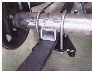
21 The shackle plates bolt up with the lower shock mounts facing the centersection and toward the rear. The U-bolts are not completely tightened up yet, as we still need to accurately set the pinion angle before tack-welding the spring pads to the housing.
