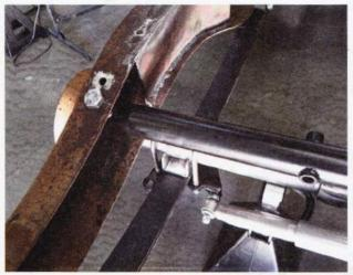
The crossmember may also be welded in place—just be sure placement is dead-on (shocks mocked up and so on) before doing so.
