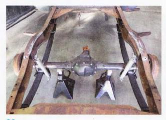
22 Next, the supplied gas shocks are bolted up in preparation of installing the tubular crossmember.
