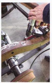
24 We marked our framerail accordingly and drilled the upper holes first.
