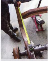
23 The measurement for locating the crossmember is taken off the rearmost bed mounting hole, which according to TCI Engineering is 281/8 inches. When locating, the important things to consider are shock angle and ensuring the differential cover will not contact the crossmember upon full suspension compression.
