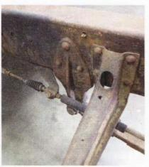
**03-04** Rivets abound—roughly 20 of them need to be gotten rid of: those retaining the e-brake cable housings are optional, as they can be reused with the adapted e-brake cable from CPP, but the forward leaf-spring hangers and the rear shackle brackets must go.
