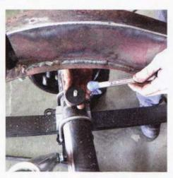
30 Last step before tacking the spring pads in place: setting pinion angle. Basic rule of thumb is to keep the up angle of pinion yoke "parallel to" (not directly in line with) that of the transmission tailshaft/engine crank centerline.
