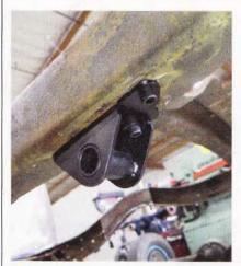
14 The forward mounting hole (nearest the cab) for the shackle bracket requires the bolt to be installed from the top; the rear two install from beneath, as shown.
