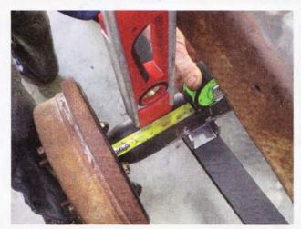
**20** The rearend is then centered on the springs and within the framerails—the latter of which is checked (and cross-checked) for squareness in the process.
