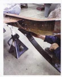
17 With the rearend prepped and all brackets securely mounted, the new 21/2-inch leaf springs were installed into the hangers.
