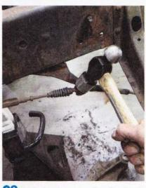
On the brackets mounting directly off the bottom side of the framerail, we simply ground the heads flush and hammered or pried the brackets off.
