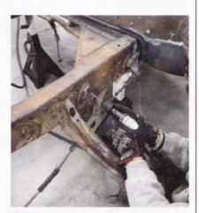
**06** The new leaf-spring bracketry bolts directly into existing frame holes—the very holes currently occupied by rivets, thus the need to "carefully" remove the rivets so as not to compromise the holes.
