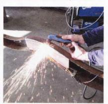
15 As you may or may not have noticed, a prior frame boxing had been attempted. So as not to create a ton more work for ourselves, we simply hacked off the top portion protruding above the 'rail, rewelded flush with the frame, and cleaned up with a grinder.
