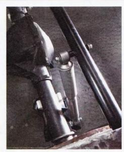
29 Same / thought process goes for locating the bumpstops-in other words, do not place them directly above the axle tubes, rather, slightly behind. (The tape on the wrench is aiding holding the Nyloc nut blindly from behind the boxing plate.)
