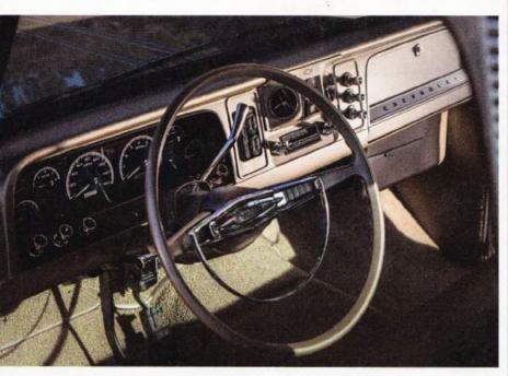
gauges. The universal six-gauge set is mounted in place of the stock instruments. In the center of the dash, electronic controls for the AccuAir air suspension system replace the old slider switches for the heater—and the heater has been replaced by a Vintage Air A/C system. The steering wheel is original, mounted on a Classic Performance Products column. At Fat Lucky's in Austin, Texas, the stock C10 bench was reupholstered in fawn-colored vinyl. New old stock '62
