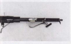
• As part of the steering upgrade we added a black, powdercoated tilt steering from Flaming River. Ours included a column shifter.
