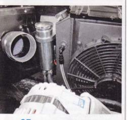
**05** To complement the LS-style power steering pump a CPP power steering reservoir with stainless steel lines was added.
