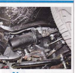
**04** Just like the original steering gear the CPP replacement bolts directly to the outside of the left framerail.
