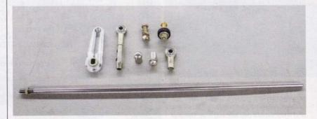
18 One of the additional changes made necessary by the steering column sway is new shift linkage. Ours came from Kugel Komponents.
