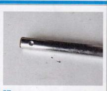
Before the U-joints are attached, the ends of the shaft should be dimpled with a drill to provide a seat for the set screws.
