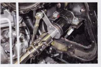
**20** Kugel's transmission arm is slotted to allow the travel of the column shifter to be matched to the gear positions in the transmission.
