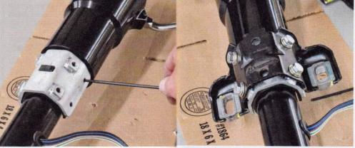
The original C10 column-mounting bracket attaches to the Flaming River column.
