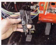
**12-13** As we pointed out in the wiring story on the same truck not long ago, the ignition switch (left) and turn signal wiring from the column plug directly into wiring harness.
