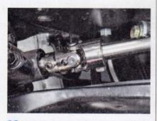
The U-joints are secured with set screws with lock nuts. A thread-locking compound should be used on the fasteners and they should be checked after the first few miles.
