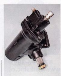
O2 To improve steering feel we installed a Classic Performance Products 500-Series steering box with a quickerthan-stock 14:1 power steering gear in our C10 Chevrolet.
