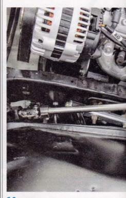
14 Another recommended update is a new intermediate shaft. Ours came from CPP and has a slip joint in the middle where the  $\frac{3}{4}$ -inch solid male and 1-inch female Double D shafts join.
