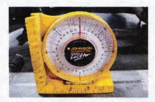
O2 Before the Scott's crossmember is tacked in place, it's checked for level and alignment.
