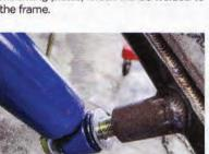
21 Next, the upper shock brackets need to be installed. First, the shocks are fully compressed and a piece of string is used to secure it. The string is tied so that the shock will remain compressed (wire can also be used). Then the compressed shock is attached to the lower control arm shock mount.
