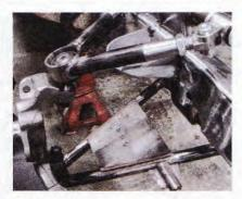
26 Each airbag will mount between the lower control arm and the upper frame bracket.
