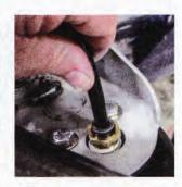
33 Once attached to the upper and lower brackets, the airbags are plumbed using the push-lock fittings.
