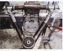
10 Here's the tubular upper control arm assembly, complete with the serviceable ball joint installed.
