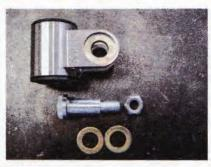
**08** Both rod ends are in turn held in place by a clevis, fastened by a shoulder bolt, with two washers on either side of the rod end and secured with a Nyloc nut.
