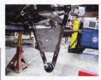
With the crossmember tacked in place, we can begin installing the Scott's suspension components, starting with the lower control arms, identifiable by the lower airbag mounts. That's the sway bar mount jutting off the front of the control arm; this should be oriented to the front of the truck.
