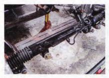
24 Installing the power steering rack in next, using two 5/8-inch fasteners to attached it to the crossmember. Note the C-notch clearance on the framerail for the tie rods.
