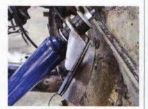
22 The upper shock bracket is then attached to the upper shock stud; note the arrangement of the bushings and washers.
