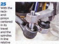
to the chassis, the outer tie rod ends can be adjusted until they slide into each steering arm and fastened with a castle nut/cotter pin, completing the basic component assembly.
