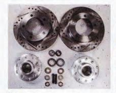
34 It wouldn't be a proper upgrade if we didn't opt for large disc brakes, so we decided to have Scott's spec our frontend using CPP's drilled and slotted 11-inch rotors and aluminum hubs.
