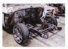
36 With the truck back on the ground and the airbags inflated to simulate ride height, our F-100 is starting to look like a proper street truck! Deflated, our truck drops the rockers nice and low.
