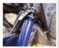
23 Per Scott's instructions, the upper mount will lays in its natural position when the shock is fully compressed. The mount will be closely pre-angled to sit in the correct position, then tack welded in place.
