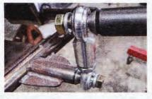
27 The sway bar requires two brackets be welded to the inside of each framerail to secure it in place. To locate these brackets, the sway bar needs to be attached to the lower control arms using the provided Heim joints and hardware.
