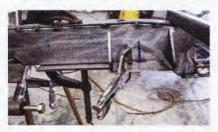
28 With the sway bar installed, it's lifted until it contacts the bottom of the frame, where a vertical mark is made on the side of the framerail. The sway bar brackets are then clamped in place using these marks. Note that the bottom of the bracket is even with the bottom of the framerail.
