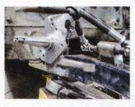
interference. Note the notch on the bottom of the framerail that gives the lower control arm plenty of clearance.
