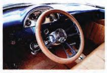
headliner; the darker leather is saddle toned and the lighter is biscuit. An aluminum insert was built into the stock dash for the Dolphin gauges. A Moon tach is mounted on the CPP steering column. The tri-spoke billet steering wheel is leather wrapped and accented with body-color paint. A B&tM shifter is housed in a custom console, built by Jess.
