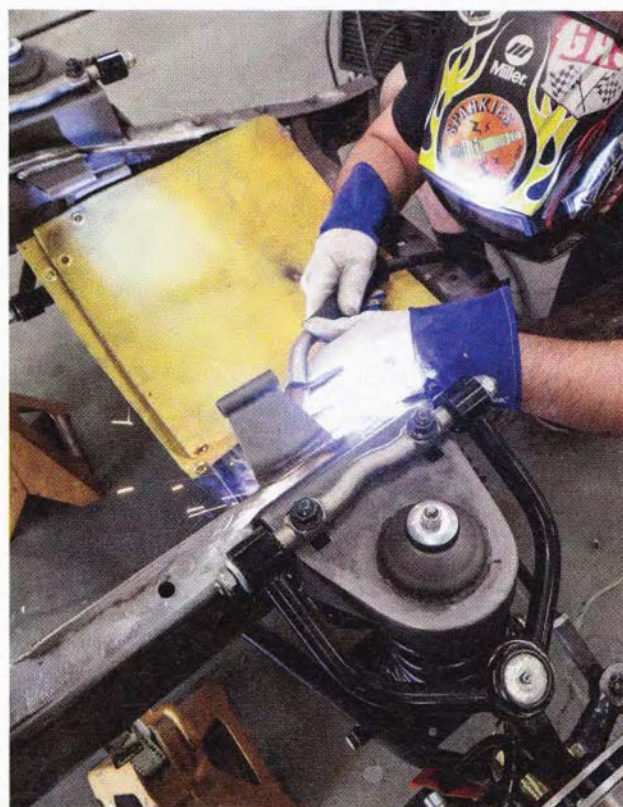
18 The mockup engine and trans, as well as the radiator and core support, were removed so that the pedestals could be properly and fully welded up.
