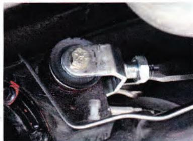
**17** | We lubed up the new bushing and tapped it into the housing until it bottomed out. We then installed the new upper control arm. To make sure we were in the ballpark, we set the length of the new upper arm the same as the stocker that was removed.
