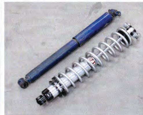
**20** | The rear coilovers were single-adjustable billet QA1 pieces and a CPP coil spring. Besides being great looking (especially compared to the stock shock), this will let us dial in the ride/handling of the Chevelle in addition to its ride height.
