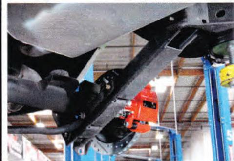
**11** | Part of improving the handling of any car is stiffening up the suspension in terms of flex. Our Chevelle actually had nicer parts than most we've seen since it was fitted with a rear sway bar and factory "boxed" lower trailing arms.
