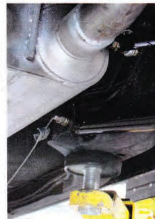
**14** | It's pretty easy to see how much stronger the new upper arm is compared to the stamped steel stocker. The other huge benefit is that it's adjustable, so we can fine-tune the pinion angle and better align the rear end.
