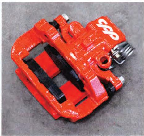
**07** With the axle reinstalled and the diff buttoned back up we then installed the new 12-inch slotted, drilled, zinc-washed rotor and bolted on the CPP caliper. The calipers had to mount forward to provide clearance for the shocks.
