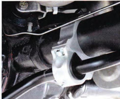
**10** | The upper brackets were bolted to the frame and then the links were adjusted and attached to the sway bar. The bar itself has three points, so the roll stiffness can be tuned for the car. For now we set it on the last hole, which is the softest.
