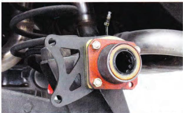
**05** And here's how the caliper bracket bolted to the housing flange. Note that the bolt at 4 o'clock wasn't used at this point in the install.
