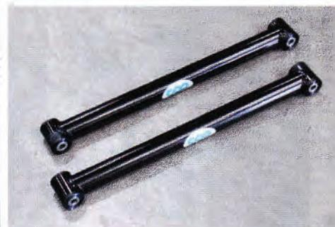
**12** | But even the upgraded, boxed GM trailing arms bend and flex a lot compared to these tubular pieces from CPP. The bars came with the urethane bushings already installed.
