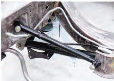
**23** CPP offers these Trailing Arm Mount Adjustable Braces (PN 6467TAMB, \$89). We couldn't add them due to our mufflers being too far back, but if you have space, they're a great idea. Here's a picture of them mounted to one of CPP's display frames. The bar ties the rear of the upper trailing arm to the rear of the lower trailing arm and adds a lot of chassis stiffness.
