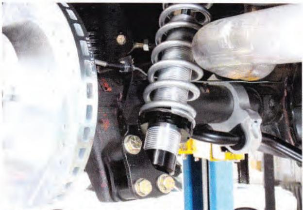
**21** And here's the coilover shock mounted under the Chevy. We lucked out and just managed to clear the exhaust, but keep in mind that the coilover conversion does take up a bit more space than a standard shock.
