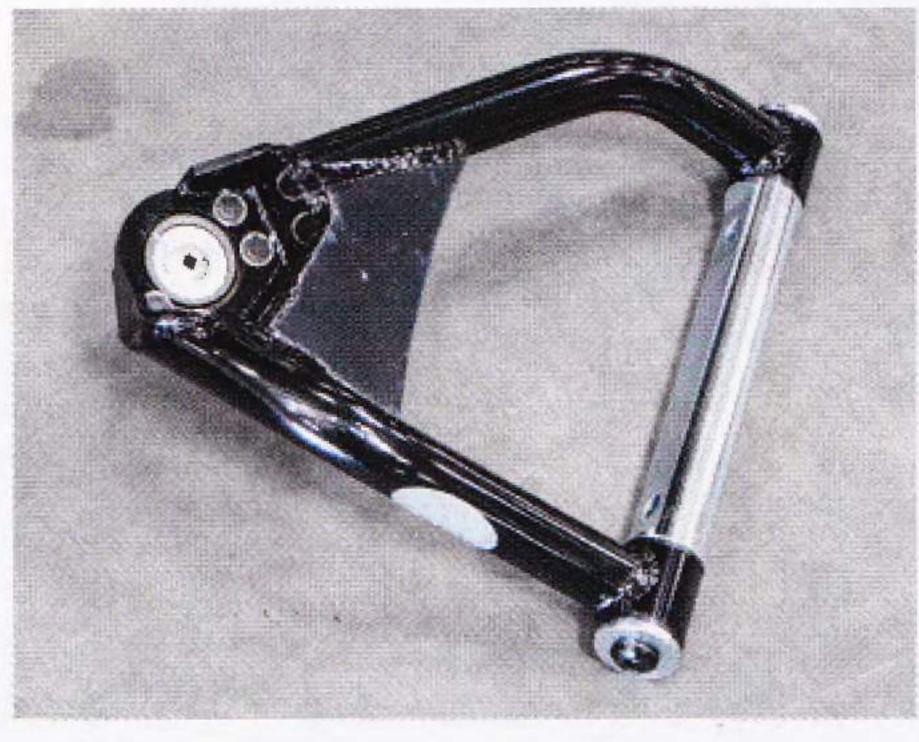
even under stress. They come preassembled on new billet chromoly 4130 cross-shafts and pivot sleeves. These sleeves capture both sides of the bushing, unlike the stockers that are only retained on one side. As a result, they're much stronger and better resist flex. As a safety measure, they incorporate an interlocking shaft and sleeve design so that the bolts can't work loose. The fact that they came with new ball joints already installed saved us time.
