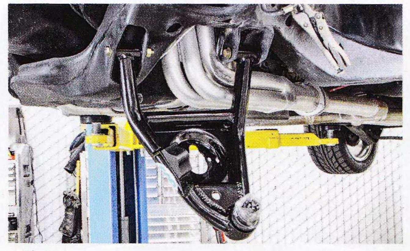
First to go on, with the supplied Grade 8 hardware, were the new tubular lower control arms. The TIG-welded arms came pre-assembled with new bushings and Moog ball joints. CPP designed the arms so that the same part will work for traditional-style coil springs as well as their coilover shocks. This is a nice feature for those who want to start with springs and upgrade later.
