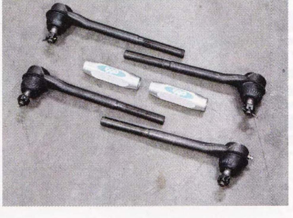
kit included inner and outer tie rods, pitman arm, idler arm, and centerlink.
