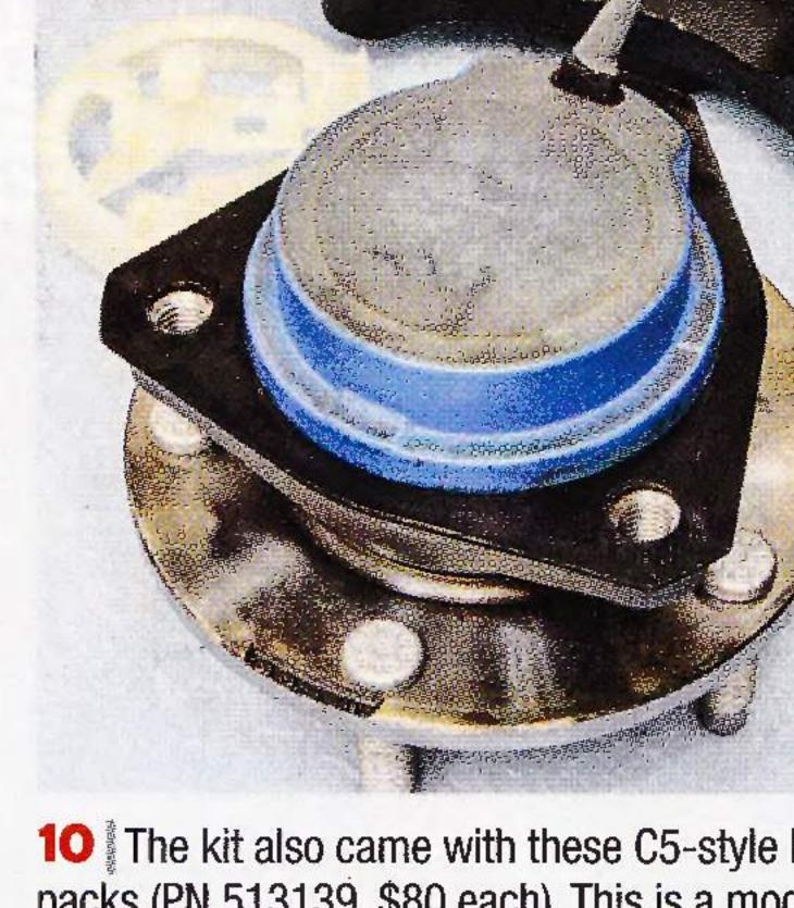
The kit also came with these C5-style bearing packs (PN 513139, \$80 each). This is a modern sealed bearing that simply bolts to CPP's new C5-style spindles. They don't change the track width at all, and even have the ABS wheel-speed sensors if you want to try going that route.
