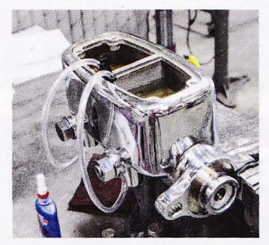
The Stage-IV kit came with CPP's slick MCPV-1 master cylinder. Besides being all shiny and chrome, the 1-inch bore master had a built-in adjustable proportioning valve. Before installing, we bench-bled it with the kit supplied by CPP.
