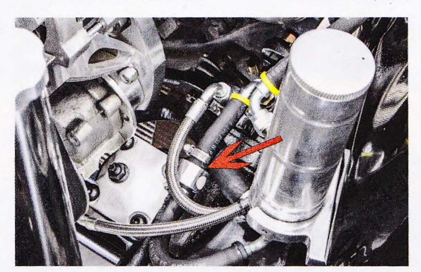
22 Since the Hydra Stop uses power steering fluid pressure, we had to rework our power steering hoses. We also added a small Magna Pure filter (red arrow) (PN 20-0038F, \$20) after the Hydra Stop unit to make sure no contaminants would clog the unit. The plumbing was made easier with CPP's stainless hydraulic brake assist hose kit (PN HAHK-S, \$199).
