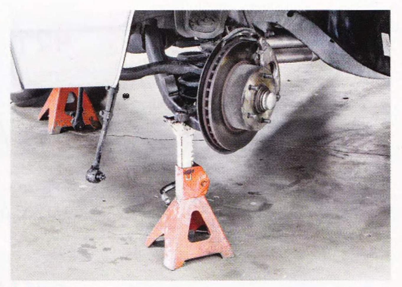
O4 It was then time for the part we hate, namely, removing the coil springs. We couldn't get our spring compressor in place so we used a jack stand and the lift to slowly raise the car and relieve the tension on the coil springs. There are many ways to skin this feline, but just make sure to be careful since there's a ton of stored energy in the compressed spring. Once the spring was gone, we went ahead and removed the stock control arms, sway bar, and worn steering bits.
