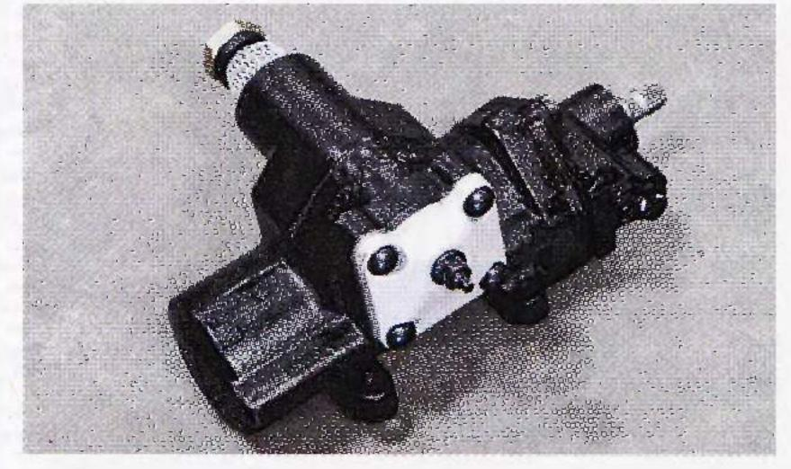
14 The replacement box was a CPP 14:1 close-ratio 500 box (PN CP50004, \$379). Having good steering response is critical if you want to improve the handling and feel of an older Chevy, and it's one of the easiest upgrades you can do. The CPP kit came with an aluminum top cover.
