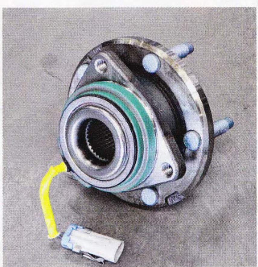
For cars that are going to be pushed hard (or extremely heavy cars), CPP recommends upgrading to their high-performance SKF hub bearings (PN BR930544, \$858). These are a lot more robust and will better withstand side loading compared to the standard bearing packs. The upgrade cost is \$429.
