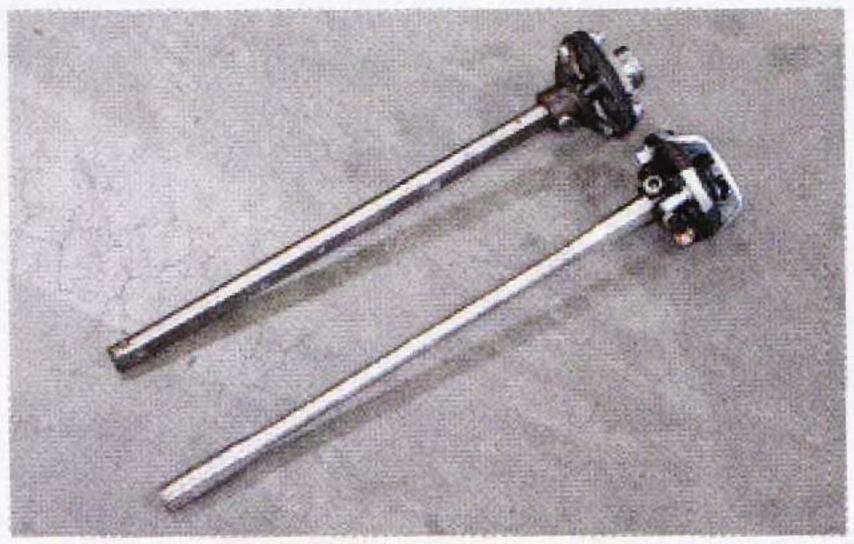
The headers on our big-block were pretty close to the factory steering shaft so we gained a bit of room by using CPP's Max Clearance nickel-plated power steering shaft (PN CPMAX-KN, \$139), which included a coupler and a new rag joint.
