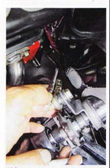
16 Now that we've achieved plane adjustment sufficiently, we just need to trim the length accordingly. When doing so, make sure both shift levers are in the Park position.
