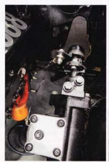
**21** Install complete: automatic transmission and tilt column joined successfully.
