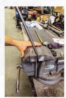
14 With the rod mounted in a vice, a length of pipe is used to form the two bends.
