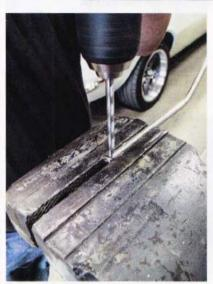
18 Trimmed with a cutoff wheel, the upper end of the rod is then marked and dimpled with a drill for the hex connector set screws.
