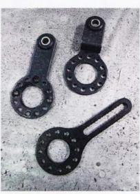
O3 CPP's Classic Fit tilt column, to which we're about to install the linkage kit on, comes standard with a flat shift lever as well as a doglegged version—both offering multi-position mounting options. Also shown is CPP's "adjustable" shift lever (bottom), which cannot only be clocked in various positions, but its serrated/slotted arm allows for more linkage adjustment as well.
