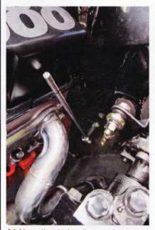
11 In an attempt to keep the connector perpendicular to the end links (an angle connection could be made, but travel would be affected), we'll need to put a couple of doglegs in the rod.
