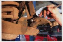
For the spindles, we used a 3/4-inch box wrench top and bottom. If you don't have access to a ball joint tool, you can also try using a hammer and some hard blows on the spindle edge to more or less "pop" the joint loose. We were lucky; the spindle practically fell off.
