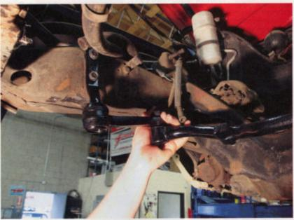
CPP's kit comes with a new idler arm, so we went ahead and painted that with the factory center steering bar. We bolted up the new arm with a 5/8-inch socket and an 11/16-inch wrench. From there, Miramontes attached the center steering bar with its associated nut and fastened it down with a 9/16-inch wrench.
