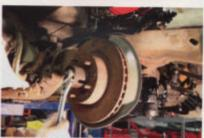
For the time being, Miramontes reinstalled the factory rotors by setting the rotor back onto the spindle. Using an adjustable wrench, he fastened the nut into place and finished it off with a cotter pin and the dust shield.
