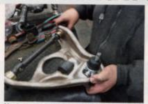
Next we needed to install! CPP's new bushings, ball joints, and bumpstops. The ball joints were a cinch and bolted in with new hardware, and a 7/16-inch wrench was used to tighten them down. The new ball joints also require a special installing tool. If you don't have access to one, we recommend getting a rental from your local hardware store.
