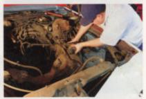
Miramontes dove into the engine bay and began unbolting the upper A-arms. He used a 15/16-inch socket and wrench on both sides to remove them. He took note of how many shims were on each side and set those aside. Alignment will have to be done once the new parts have been installed.
