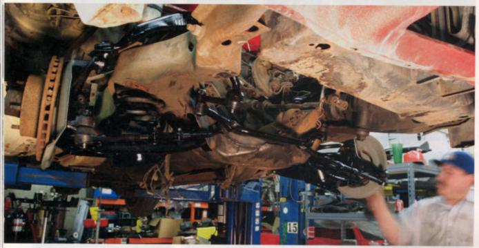
At one time or another we all end up taking our rides for granted and paying the price. Case in point, when vehicles sit idle for a while you can kiss your joints and bushings goodbye. Without the movement of the car's suspension, grease
