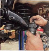
The spindles were next; we started by placing the lower ball joint into the bottom of the spindle. Using a jack, we pushed up the lower A-arm until the upper portion of the spindle met the ball joint from the upper A-arm. We fastened the spindle down into each A-arm using a 3/4-inch wrench. Finally, we attached the tie rods into the ends of the spindle and used a 9/16-inch wrench to tighten each nut.
