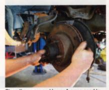
Since the upper and lower A-arms need to be disassembled, we first had to remove the rotors from both sides. Miramontes removed the small grease cover and the cotter pin and, using an adjustable wrench, removed the spindle nut and took off the rotor.
