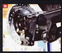
One upgrade we opted for was CPP's coilover conversion kit (PN PTK-RCOILOVER-SA, \$229). Here you can see the main shock bracket assembly. The larger spacers went between the two plates while the short ones went between the rear plate and the existing shock mount. The system utilized the existing shock mounting hole, but we had to drill a hole for the upper bolt. If you look closely you'll notice that the plates have a slight bend in them. This adds a ton of strength to the finished assembly.
