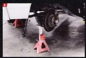
It was then time for the part we hate, namely, removing the coil springs. We couldn't get our spring compressor in place so we used a jack stand and the lift to slowly raise the car and relieve the tension on the coil springs. There's many ways to skin this feline, but just make sure to be careful since there's a ton of stored energy in the compressed spring. Once the spring was gone we went ahead and removed the stock control arms, sway bar, and worn steering bits.
