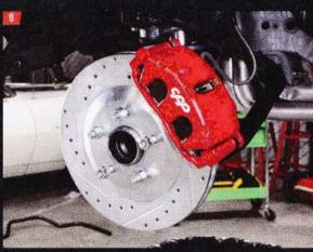
With the new control arms installed the rest was crazy easy to do. The main reason for this was that the front spindle, hub, steering arm, and brake parts came completely preassembled from CPP. Even the brake pads were installed, so all we had to do was toss the whole deal between the control arms and secure it in place with castle nuts and cotter pins.
