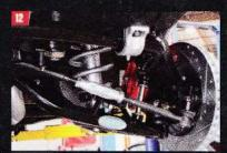
Here's the completely assembled left front suspension system. You can also see the new 1.25-inch hollow sway bar and CPP's new 2.5-inch aluminum sway bar mounts (PN FBM25-M285, \$69 each) which look great and are stronger than the stamped-steel versions.
