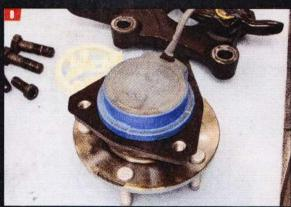
The kit also came with these C5-style bearing packs (PN 513139, \$80 each). This is a modern sealed bearing that simply bolts to CPP's new C5-style spindles. They don't change the track width at all and even have the ABS wheel speed sensors if you want to try going that route. For cars that are going to be pushed hard (or extremely heavy cars) CPP recommends upgrading to their high-performance SKF hub bearings (PN BR930544).
