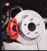
We were then able to install the new 12-inch slotted, drilled, zinc-washed rotor and bolt on the CPP caliper. The single-piston floating calipers (with integrated parking brake) had to mount forward to provide clearance for the shocks.
