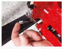
23 Install the new parking brake cables onto the caliper by sliding the end through the cast bracket in the caliper and attaching it to the parking brake lever. Adjust so that all slack is taken out of the cables. Secure with the clip provided.
