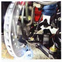
11 Torque the caliper mounting bolts to 100 lb-ft with your torque wrench and your 7/8" socket. Spin the rotor to make sure you do not have any contact, the rotor spins freely, and the brakes pads are not binding too tightly (slight drag is okay).
