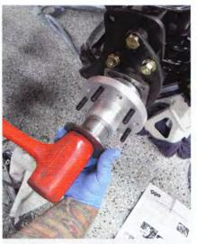
**6** Install the grease cap by tapping in with regular hammer and socket, or a rubber mallet and steel tubing, as we did.
