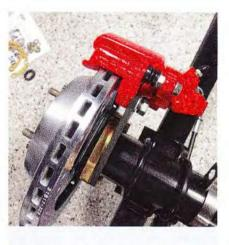
**21** Once the calipers fit correctly, securely tighten up all mounting bracket and caliper hardware, using lock washers wherever necessary. Spin the rotor to ensure even pad contact with no binding.
