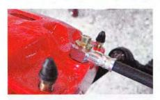
12 Install the new brake hoses on the calipers with the new crush washers (one on each side of the hose fitting) and new brake hose bolt. Install the other end to the brake lines. Tighten with the 11mm flare nut wrench.
