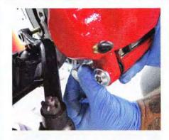
**10** The lower mounting bolts will only go in with the steering arm loose and out of the way, as shown.
