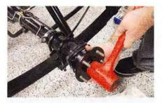
**16** Carefully re-install the axles, sandwiching the bearing spacer plate between the stock retainer and the axle housing flange.
