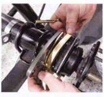
**20** The shim(s) will go between the two caliper bracket halves; the bolts must be completely removed in order to install them.
