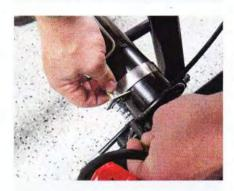
22 Install the brake hose tabs and clips onto the new brake hoses. Connect the brake hoses to the hard lines. You may need to modify the hard lines to get a proper or clean fit. Secure the brake hose tabs around the axle with the tab clamp. When everything is in place, using your 10mm flare nut wrench, tighten the ends starting with the hard line. Tighten the bolt against the crush washers in the caliper.
