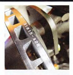
The rotors are marked Left and Right (also indicated by the holes/slots flowing towards the rear).
