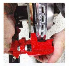
19 Slide the rear caliper assemblies over the rotors, as if you were going to install them. If they go on with no bracket interference, no shims are necessary; if not, as shown here, remove calipers and rotors and add required number of shims to relocate bracket enough to fit caliper.
