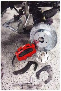
The Classic Performance Products (CPP) Big Brake four-wheel disc setup with zinc-washed 13-inch drilled rotors, dual-piston calipers, and forged aluminum hubs up front and 12-inch drilled rotors (also zinc washed) and single-piston calipers on the rear with integrated E-brake setup is the easy answer. We'll show you how to install the whole package (which works with
