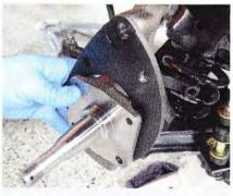
1 Start at the front by installing the new two-piece brake caliper brackets on the spindle. If replacing spindles, you will need to do so now—a spring compressor will be necessary to safely perform this step. The main bracket mounts on the wheel side of the spindle on the top, and between the spindle and the steering arm at the bottom in the rear.
