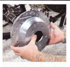
18 Install the rotors onto the axles; hold in place with lug nuts. As with the front, the rotors are marked (L/R) for orientation.
