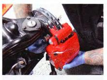
**9** Install the calipers on the caliper mounting brackets. The calipers install with the bleeder pointing upward or you will not be able to properly bleed the brakes. The caliper ear goes between the rotor and the bracket and mounts with the two caliper mounting bolts, flat and lock washers that are provided in the kit.
