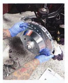
7 Install the new rotors on the hubs.
