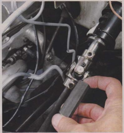
CPP's steering column kit includes a cut-to-fit intermediate shaft to connect the steering box and rag joint to the column at the firewall. We needed to trim about 2 inches from the intermediate shaft in our chop saw, then we were able to button the whole assembly up.
