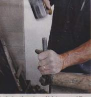
Replacing the universal joints seemed like a good idea, especially considering they looked as old as the truck is. That process begins by driving out the old joint.
