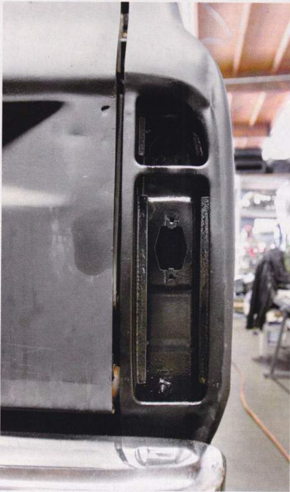
While the wiring was out, we took the opportunity to clean some of the grime behind the rear lights and treated the area with Eastwood's Rust Encapsulator.
