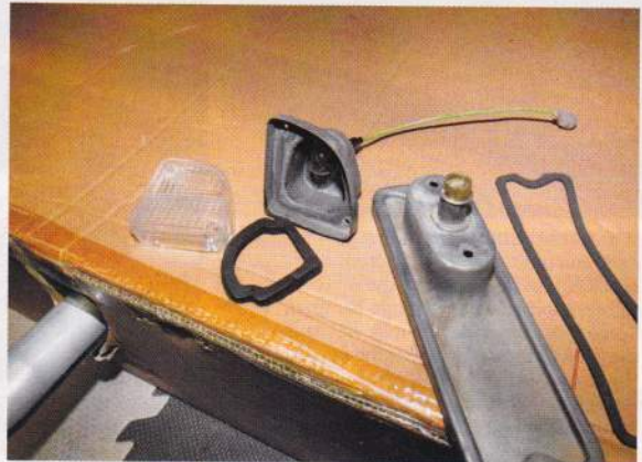
We also cleaned the lamp sockets with a wire brush and reassembled them with new back-up lenses from Rock Auto and gaskets from Brothers Trucks. We recommend using dielectric grease on the bulb receptacles. It protects electrical connections from corrosion, which is especially useful in an area like this as it becomes contaminated with dirt and moisture over time.
