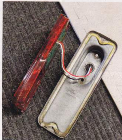
We also cleaned the lamp sockets with a wire brush and reassembled them with new back-up lenses from Rock Auto and gaskets from Brothers Trucks. We recommend using dielectric grease on the bulb receptacles. It protects electrical connections from corrosion, which is especially useful in an area like this as it becomes contaminated with dirt and moisture over time.
