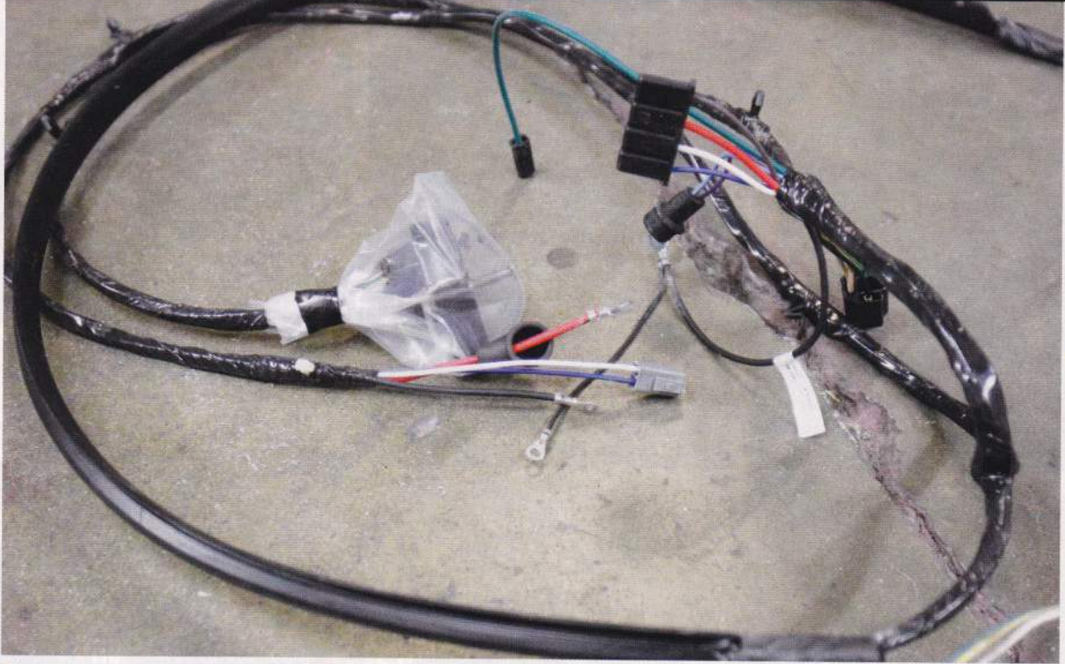
The new harnesses are exact replacements of the originals. This is the front engine-compartment harness, which includes the correct bulkhead connector and plastic channel that runs across the radiator core support to power the headlights and turn signals.
