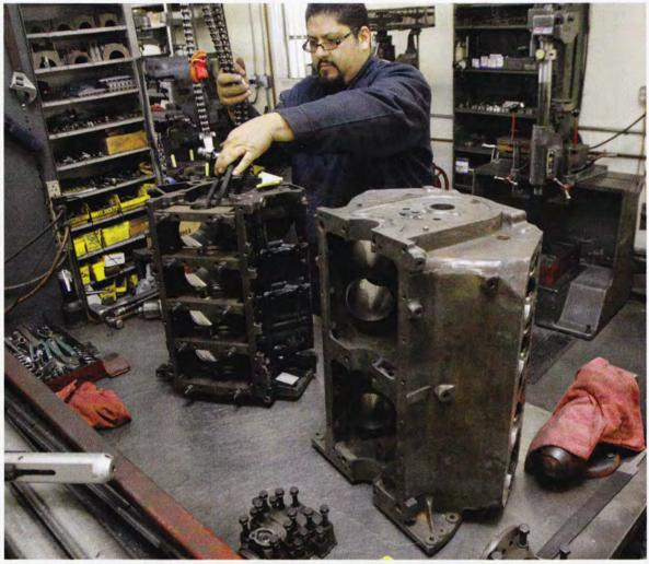
With four-bolt mains and cross-bolted main caps, it's easy to see why a stock LS engine block is stronger than previous small- and big-block Chevys, and especially the Flathead block to the right of it.
