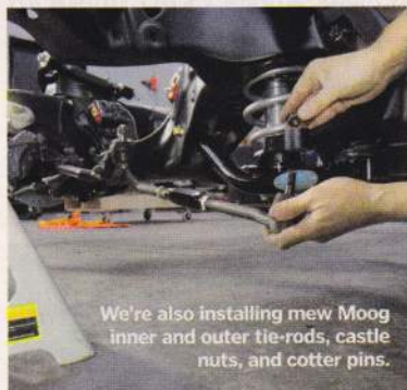
Here's the new billet tie-rod adjuster, complete with jamb nuts on either side, which will make alignments much easier.
