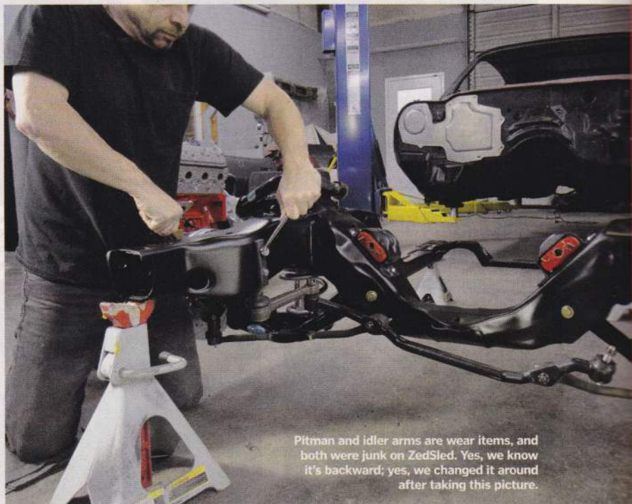
We're also installing mew Moog inner and outer tie-rods, castle nuts, and cotter pins.
