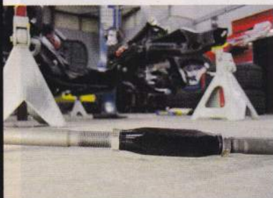
Here's the new billet tie-rod adjuster, complete with jamb nuts on either side, which will make alignments much easier.
