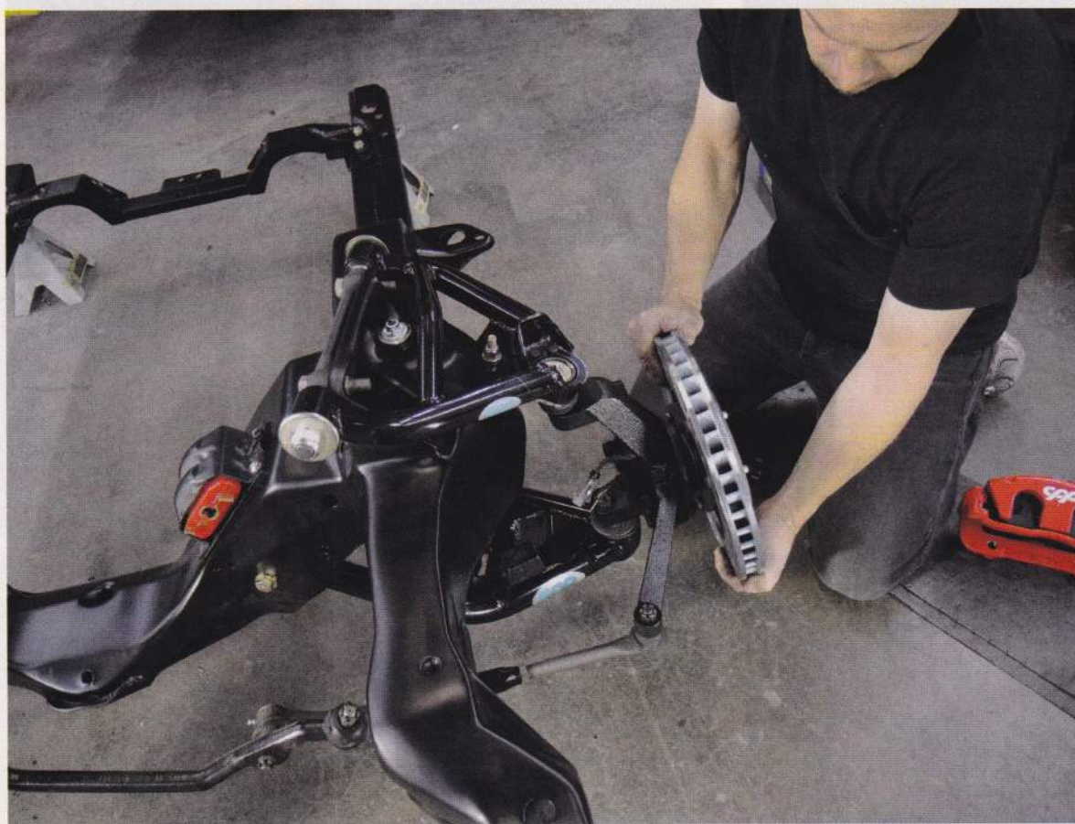
The colossal 13-inch Corvette rotors slip over the C-5 hubs before the calipers are attached. Note: You'll be switching to an M12 thread size with the new hubs, so make sure you have the correct lug nuts if you're doing this swap.
