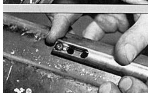
Check the position of the new holes by sliding the housing into the tailgate. Also check the holes by inserting the mounting screw through the housing and into the hole. You can see how the other two holes become the outer edges of the area needed to create the sliding knob gap.
