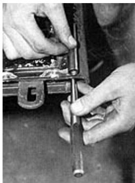
The first thing to do is remove the locking pin and spring by removing the plastic knob. Then, position the housing by centering it within the area of the upper tailgate lip. A center punch is then used to mark the center of the pin.
