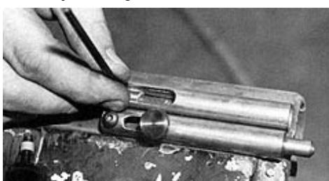
Once the hole positions are determined, the mounting screw hole is drilled with a 3/16-inch bit, while the two other holes, which will be cut out in-between and serve as the slide gap, are drilled with a 1/4-inch bit.
