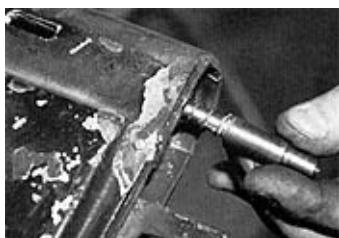
Reinstall the spring on the locking pin, along with a small amount of lithium grease, and insert it in the housing.
