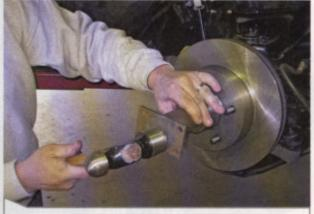
Craig showed us this little trick for installing grease caps without bashing them in with a hammer. Take a piece of tubing that fits over the cap and use it to seat the grease cap.
