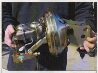
Luckily, CPP has a variety of master/booster combos available, including this very nice stock '67-72—style unit that CPP makes. It mimics the stock dimensions and operation to a "T" and can be ordered for a disc/drum or drum/drum setup depending on your needs. The 11-inch booster is gold cadmium—plated just like the originals and looks great in a driver or resto/show truck.
