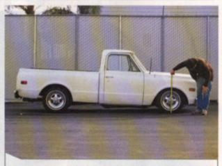
With the 2 ½-inch dropped spindle and 2-inch dropped coils in the front, the C-10 measures roughly 26 inches from terra firma to the top of the front wheelwell. Basically, it's on the bumpstops up front, which isn't for everyone, but a simple coil spring change would give a bit more clearance. The back is going to come down in the near future—don't worry.
