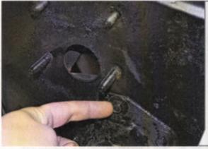
This is where the fifth mount goes on the firewall. Since this was originally a manual disc/drum truck, there was no booster bracket on it until someone made the one to mount the junkyard booster/master. The fifth mount is also a little offset from the plane of the other four mounts, which CPP's bracket accommodates perfectly instead of just mashing it down like many others out there.
