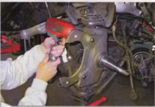
The brackets to mount the stock GM calipers are easily bolted to the spindle. These brackets have a slight bend in them to locate the caliper on the rotor properly. The bend should be toward the outside.
