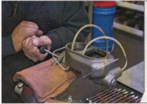
Before installing the booster/ master assembly, the master cylinder was removed and bench bled. Bleeding the air out of any new master cylinder like this is highly recommended since it is much easier than trying to push any air bubbles all the way to the wheel cylinders or calipers to be released.
