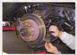
For grins, we put back on the old stock brakes to pull some measurements since we are also going to check out CPP's other brake options. With the truck back on the ground, the ride height didn't change a bit from the 2 ½-inch dropped spindles that were in it before, and they also pulled the tire in about a full inch on each side! These are the brakes that we recorded a best 60-0 stopping distance of 172 feet, which is in the not-so-great range.
