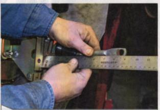
The pushrod needs to be set to the same length as the old one. This is measured from the back of the mount to the pivot hole. Once this is set, tighten the jam nut. The CPP reproduction booster/master bracket is done just like the original with its unique fifth mount seen down by Craig's right hand.
