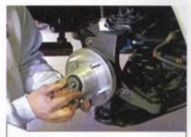
Next, the hub gets fresh bearings, grease, and inner grease seal before going on. CPP uses the large truck bearings in their hubs, which only makes sense, but many other companies use smaller passenger-car bearings for their big brakes.
