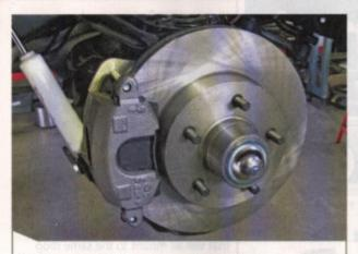
Here's the complete 12-inch stock-type disc brake kit installed. If you don't need the whole kit, each piece is available a la carte. Again, we put the truck back on the ground to take some measurements from the factory brakes, and these brakes didn't change any of the dimensions—which is a good thing!
