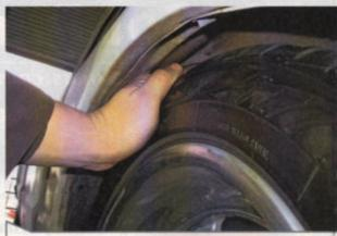
To illustrate the results of my non-scientific test (aside from the tape measure), here's the truck at the same height while being pushed down on. Now I can get my whole hand up between the 18-inch wheel and the inner fender—and I have big hands.
