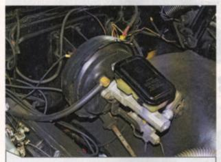
We're going to turn our attention to the master cylinder/booster combo in the truck for a little while. My truck was originally equipped with a manual disc/drum brake system. Somewhere along the line it got switched to power-assist with parts from the junkyard. This wasn't a bad thing, but it looks like ... well, um, not the best.
