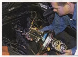
Now the whole assembly can be put in its rightful place. It helps to have someone on the inside of the cab to guide the pushrod back to its location. Don't forget to secure the rubber boot seal in the firewall, too.
