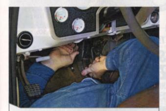
One of the first things that needs to be done to remove the old booster/ master assembly is to take the pivot bolt out of the brake pedal that connects it to the booster pushrod under the dash.
