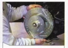
Now the impressive drilled and slotted 13-inch rotors can go on. These babies slide right onto the hub; a lug nut threaded on will help hold the rotor while installing the caliper.
