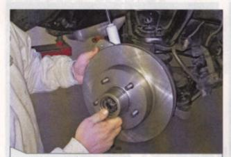
If you don't have disc brakes on your truck or need to replace your old factory ones, CPP can do that too in either a five- or six-lug rotor. These replacement disc brakes are installed just like the OE brakes and come with new wheel bearings and seals and can be used on stock or dropped spindles.
