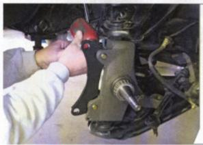
Now it's time to make good on the Modular-ness of CPP's new spindles. The spindles were stripped back down and the caliper brackets for the 13-inch discs were installed. These are flat, so there is no left and right.
