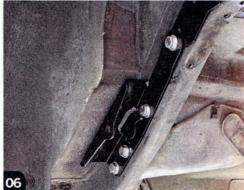
O2 Following the instructions, we measured from the rear leaf spring mount forward 18.75 inches and made a mark. It's important that the kit be installed square, although if you're off a touch it can be adjusted for with the links.
