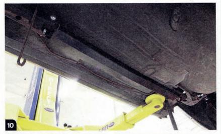
O7 We then pulled the back seat, drilled three holes, and bolted the plate through the floor using another "sandwich" plate on the inside of the car. This was repeated on the passenger side.
