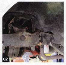
Nothing remarkable here, just 45-year-old stock suspension parts along with some tired drum brakes. Before tearing the car apart, we baseline tested the Camaro's handling and stopping. We won't give away the gory details until part two, but let's just say it wasn't very good.
