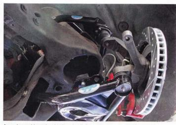
A mock-up without the shock and coil shows you how much cleaner than stock this brake setup is.
