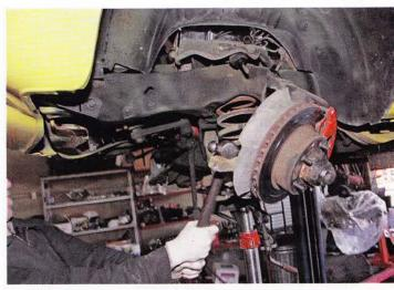
Once the castle nuts are removed, it takes some smacks with a hammer to jar loose the factory brake assembly.
