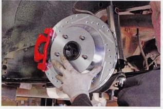
CPP's Big Brake kit (PN 6869RWBK-P12) for the rear is a popular upgrade in GM vehicles. It uses a cool caliper design that has the parking brake integrated into the caliper itself.
