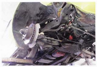
Here's your average second-gen Camaro front suspension and steering; just stamped-steel factory components and greasy hardware. Replacing the cracked and worn bushings alone would tighten things up, but we aimed to do more than that.
