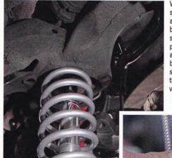
We opted for QA1 single adjustable, aluminumbodied coilover shocks for our project. You can adjust the overall behavior of the shock, as well as the ride height with these.
