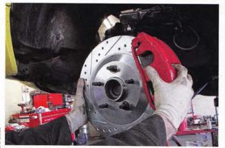
One of the many things we like about CPP's brakes is that the spindle, rotor, and caliper come all assembled. Once the upper and lowers are in place, it's just a matter of lowering the whole setup onto the ball joint.
