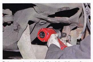
The lower control arm is attached with two bolts, which are easily removed with an impact gun at Don Lee's. Even with the bolts out, it does take some whacks with a mallet to get it free.
