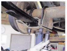
Once the new spring isolator bushings were in place, an impact gun was used to cinch everything up.
