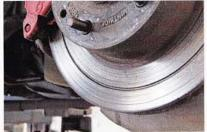
We thought we had some debris stuck between the rotor and the brake pad, but this groove is actually factory.
