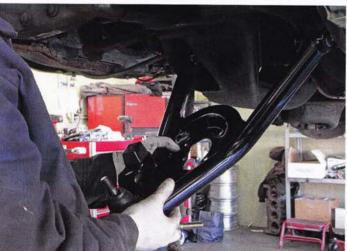
The lower control arm simply gets muscled into the factory K-frame after the urethane bushings are well lubed.
