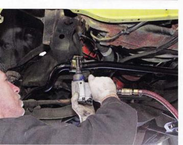
The new sway bar from CPP simply bolts in place of the stock one, using new hardware and bushings, of course.
