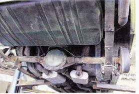
The rear suspension of the Camaro was also stock, but, like the front end, the rubber bushings were all cracked and weathered.
