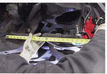
Before assembling the new steering components, the length of the tie rods must be measured and recorded. Then, the length is matched using CPP's aluminum tie-rod sleeves (PN ES2004SP-AB).
