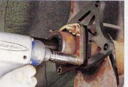
Once the C-clips were removed and the factory drum brakes were chucked, the CPP caliper brackets were installed using the new Grade 8 hardware.
