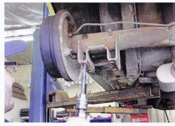
Before the new springs can be installed, the U-bolt holes needed to be widened to accept the new hardware.
