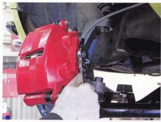
The brake system also comes with high-quality stainless braided lines that hook into the factory hard line.
