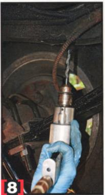
8. To line up the end links, we had to drop the chassis back to the ground and off the jacks. From there we could swing the bar and match up the ends to the frame. After marking where the end links would line up, we drilled two 3/8-inch holes into the frame.
