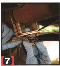
Next, we slid in our new units from Bilstein and locked them down with the factory hardware on the bottom. Don't worry about retaining the old stuff, as new bushings and nuts are included.
