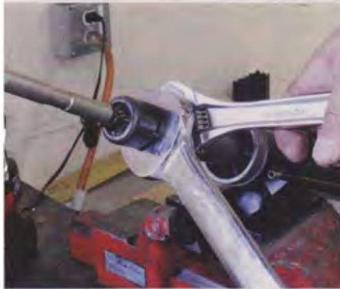
127. The original inner tie rod socket is then installed onto the rack extension, held in place ad infinitum via Loctite and a jam nut installed on the rack extension.
