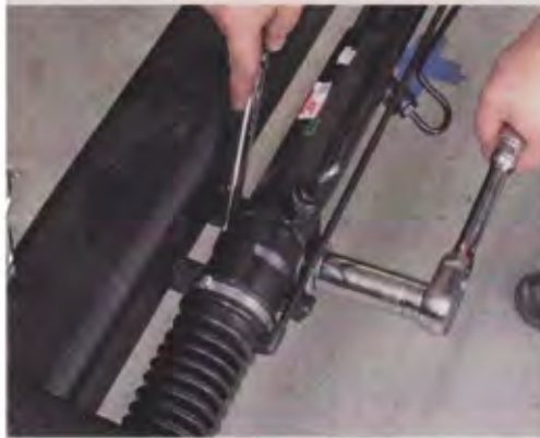
128. The rubber insulator boot is reinstalled to protect the internals of the rack and it's time to bolt the unit into place.
