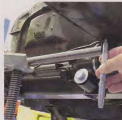
131. Next, the sway bar is pulled up against the bottom of the frame and the saddle strap mounting holes are marked and drilled.
