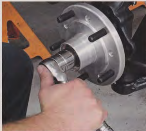
17. With the hub slid onto the spindle and the outer bearing and washer in place, the spindle nut needs to be tightened to no more than 12 ft-lb to ensure that the bearings are seated.
