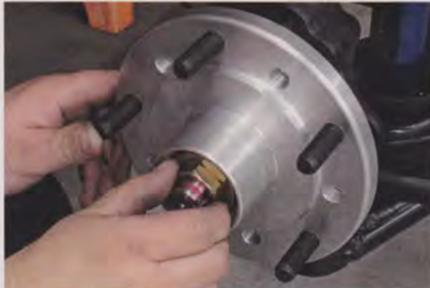
18. With the spindle nut tightened, the hub is spun and the nut rechecked for tension. If it's still tight, the bearings are properly seated and the tension on the nut relieved.
