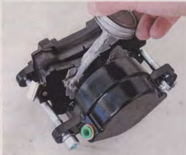
20. The next step is to install the rotors and callipers. I've had disc brake setups squeal in the past, so now I tend to err on the side of caution, liberally applying a thin coat of anti-seize to the brake pads where they contact the caliper pucks. This prevents that nasty squeal that oftentimes is the result of the pads vibrating or oscillating against the caliper and/or puck when the brakes are applied.
