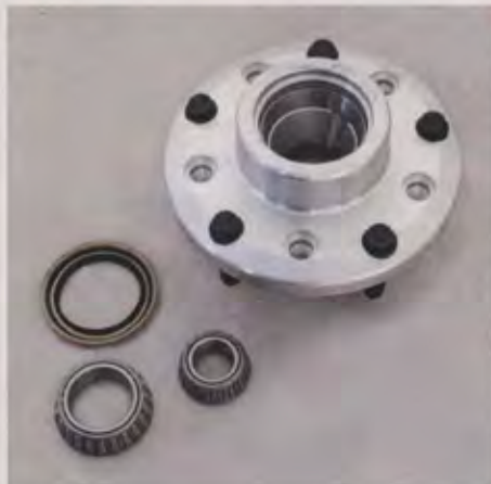
15. Here's the aluminum hub, inner and outer bearings, and seal. Note the dual bolt pattern on the hub, we're using the Ford 5x5.5-inch pattern, but CPP provides the option of using the same hub for a 5x5-inch pattern as well.
