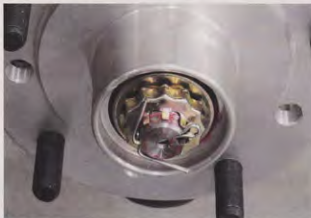
19. The nut is then hand tightened and the nut cage and cotter pin installed. A wrench is not needed for final spindle nut adjustment!
