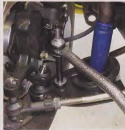
130. The last piece of the puzzle is to install the sway bar. First, the bar is installed, attached to each lower control arm via the sway bar endlink. Which, in our case, is a long fastener and a handful of rubber bushings.
